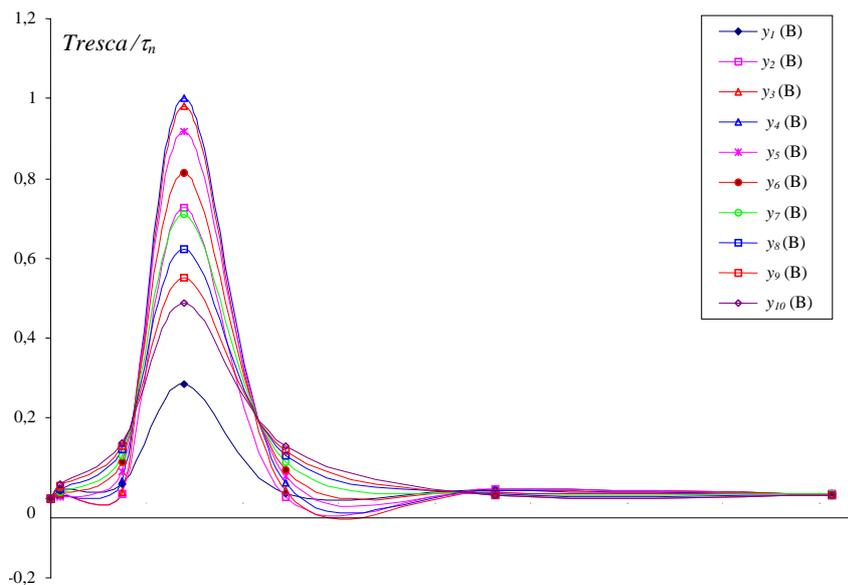
Figure 5. Normalised Tresca comparative stress cycles at meshing gears, on and under contact point B (see Figure 4b)
