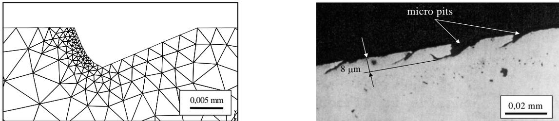
Figure 10. Numerically (left) and experimentally (right) determined pit shapes [2]
