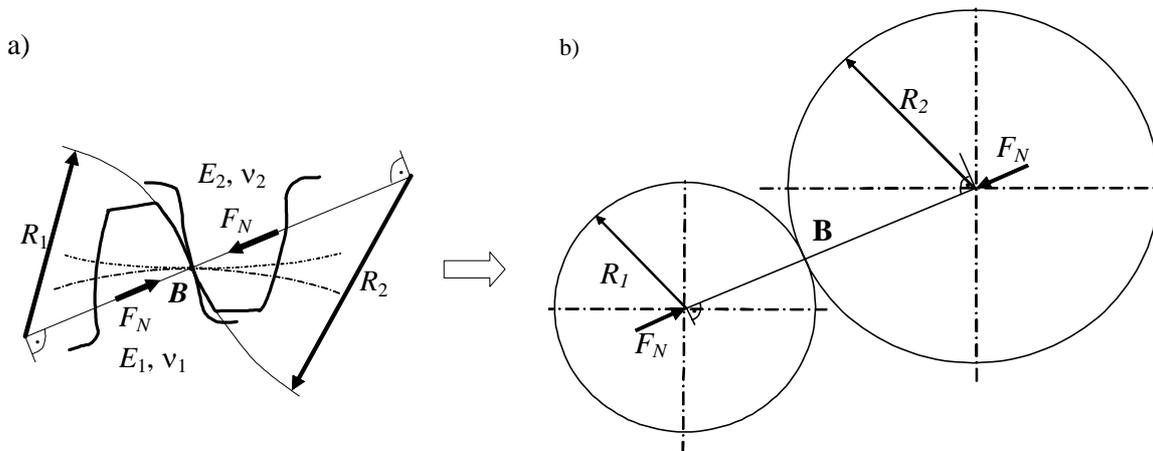
Figure 2. Model transformation of meshing gears (a) to the equivalent model of two cylinders for the meshing point B (b)
