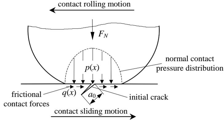
Figure 3: Orientation of the initial surface-breaking crack and contact loading.
