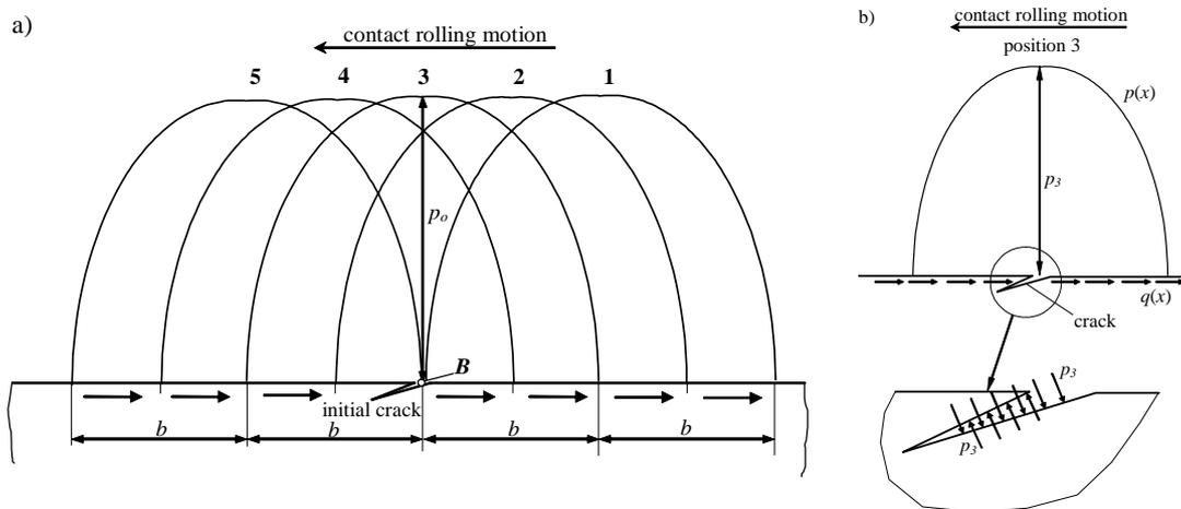
Figure 7. Moving contact loading configurations in respect to the initial crack position a) and modelling of the lubricant driven in the crack by the hydraulic pressure mechanism b)
