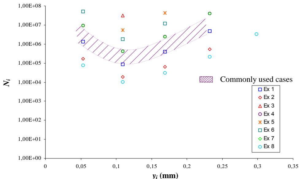
Figure 6. Results: number of loading cycles, when initial crack appear at the observed material points ( $y_i$ ) – Tresca comparative stresses,  $\varepsilon$ - $N$  analysis method
