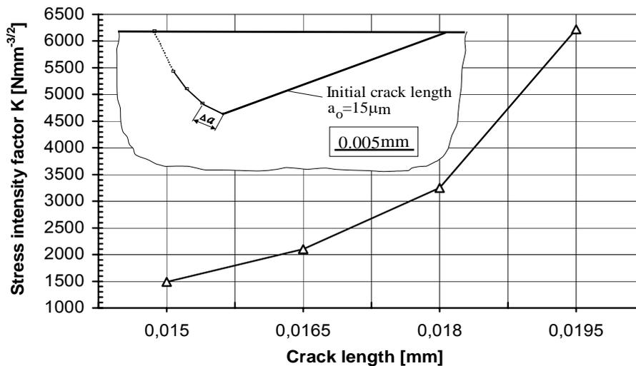
Figure 9. Stress intensity factor for initial surface micro crack propagation
