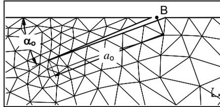
Figure 8. FE discretisation and configuration of the initial crack
