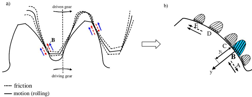
Figure 4. Moving contact loading configurations in respect to the initial crack position: meshing of gear pair (a), equivalent contact model of meshing gears (b)
