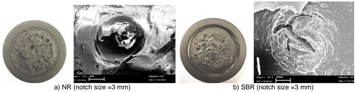
Figure 7 Damaged surfaces of the notched specimens NR a) and SBR b) in simple static tensile testing (developing of the cavities in helicoidally form and the site of the final rupture)
