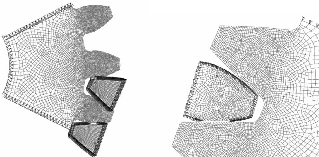
Fig.1. The pinion FEM model (two tooth pairs in contact) and a detail of the wheel FEM model (single meshed period)
