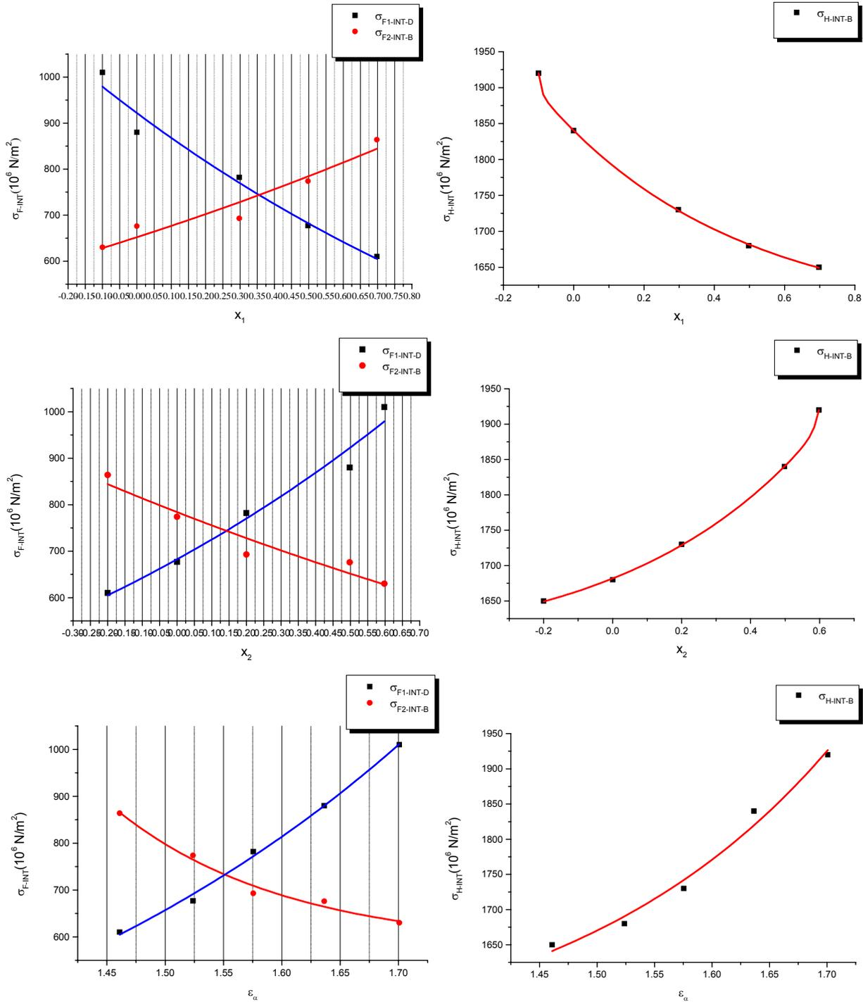
Fig.5. Diagram sets for choosing the optimal values of the addendum modification coefficients for defined gear pair series
