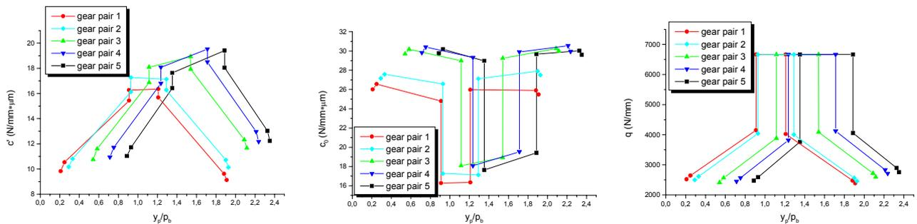
Fig.3. Comparative diagrams for monitoring the tooth stiffness and load distribution for the gear pair series
