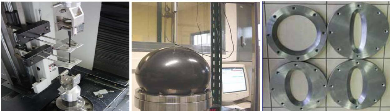
Figure 1. Equipment for (a) tensile test, (b) equal biaxial test, (c) various biaxiality ratios  $=\{1, 1/5, 1/3, 1/2\}$ .
