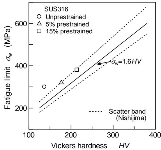
Figure 8. Relationship between Vickers hardness and fatigue limit
