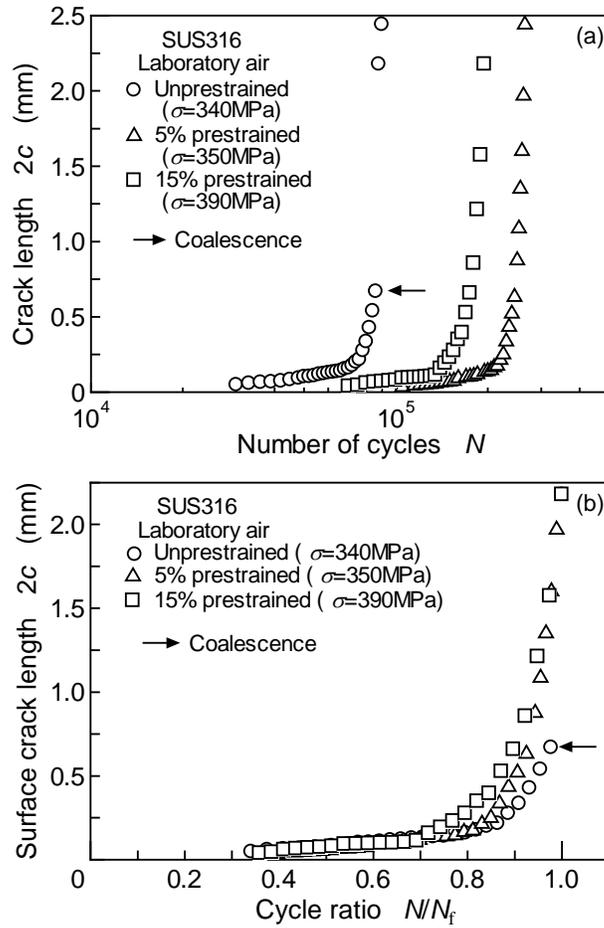
Figure 6. Surface crack length as a function of (a) number of cycles, (b) cycle ratio
