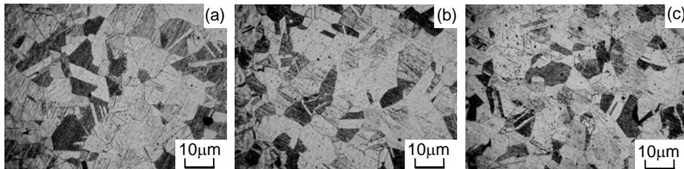
Figure 3. Microstructures: (a) unprestrained, (b) 5 % prestrained, (c) 15 % prestrained
