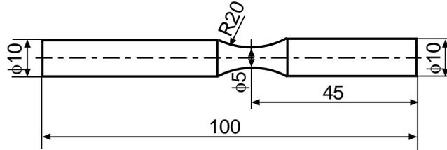
Figure 1. Configuration of fatigue specimen
