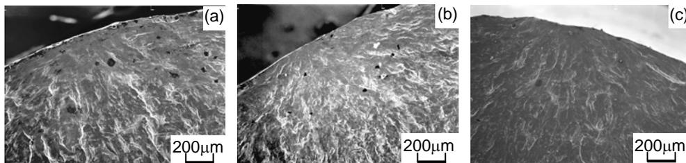
Figure 5. SEM micrographs of fracture surfaces near crack initiation site: (a) unprestrained ( $\sigma=335$  MPa,  $N_f=1.2 \times 10^5$ ), (b) 5 % prestrained ( $\sigma=330$  MPa,  $N_f=2.8 \times 10^5$ ), (c) 15 % prestrained ( $\sigma=400$  MPa,  $N_f=4.0 \times 10^4$ )
