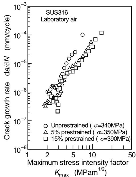
Figure 7. Relationship between crack growth rate and maximum stress intensity factor
