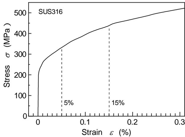
Figure 2. Stress-strain diagram
