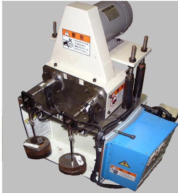
Figure 2. Dual-spindle fatigue testing machine in rotating bending
