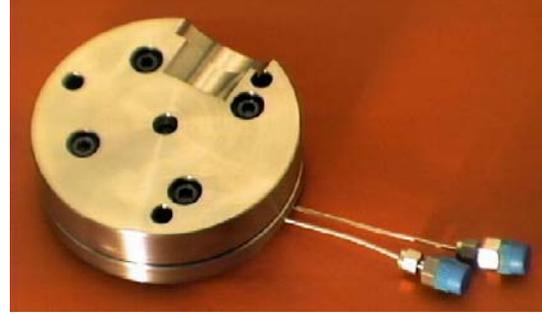
Fig. 4. Fixture/chamber for loading of the MEMS pressure sensors.
