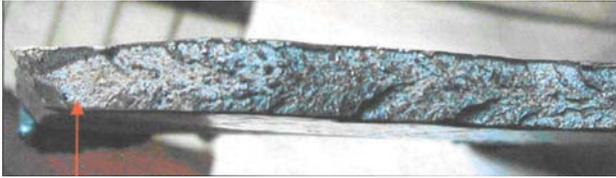
Figure 10. Fracture surface with chevron pattern
