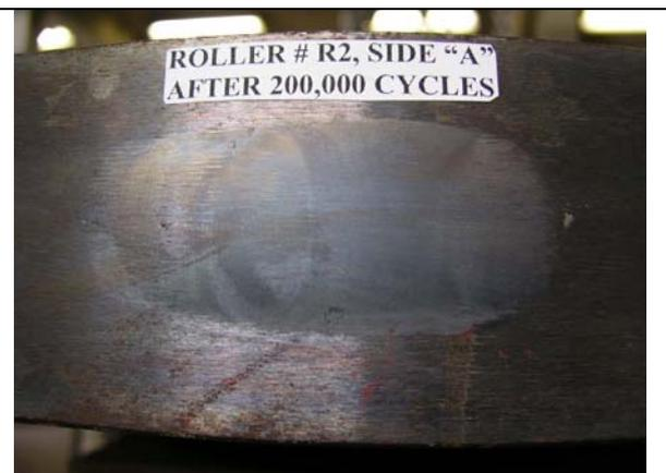
Fig. 10. Contact area of Wheel R2, Side A, after 220,000 cycles
