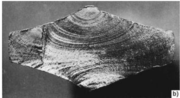
Figure 12. Macroscopic appearance of early fatigue failures showing 'conchoidal' progression markings : (a) for a propeller shaft (Gough, 1926) [27] and (b) for an unidentified component (Cazaud, 1948) [28] (Exact scales are not known).
