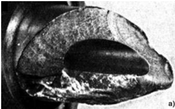
Figure 12. Macroscopic appearance of early fatigue failures showing 'conchoidal' progression markings : (a) for a propeller shaft (Gough, 1926) [27] and (b) for an unidentified component (Cazaud, 1948) [28] (Exact scales are not known).
