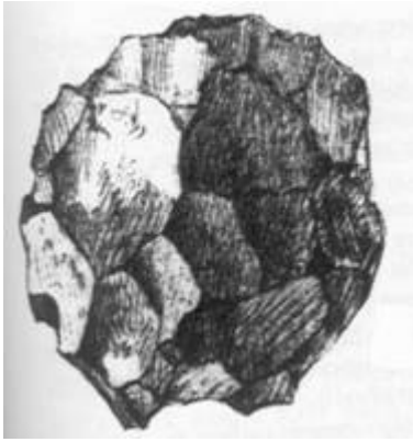
Figure 5. Photograph of a single grain of steel produced by intergranular fracture of an overheated bar (Tschernoff, 1878, reproduced in Smith, 1988 [3]).
