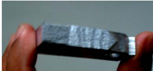
FIGURE 1 - Macro-photograph of fatigue surface. Dark bands correspond to stress ratio (R) of 0.1 and light bands correspond to stress ratio (R) of 0.7.
