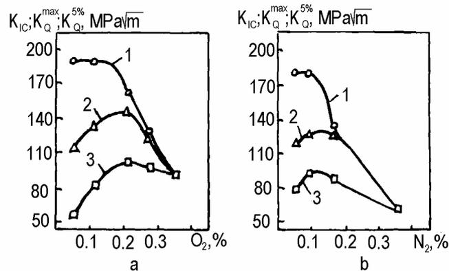
**Figure 2:** The influence of oxygen (a) and nitrogen (b) on fracture toughness  $K_{IC}$  (1),  $K_Q^{max}$  (2), and  $K_Q^{5\%}$  (3) for alloy 2V.
