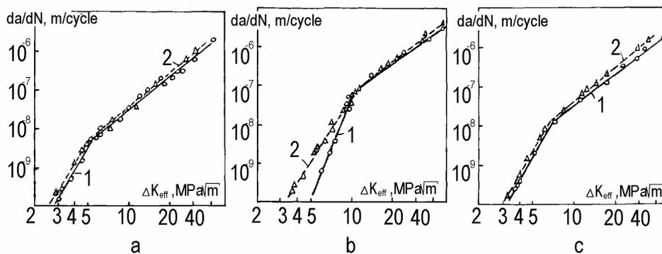
**Figure 7:** FCG diagrams in a weld and in alloy 2V with different content of oxygen in the coordinates “ $da/dN - \Delta K_{eff}$ ”. Notations are similar to those in Figure 6
