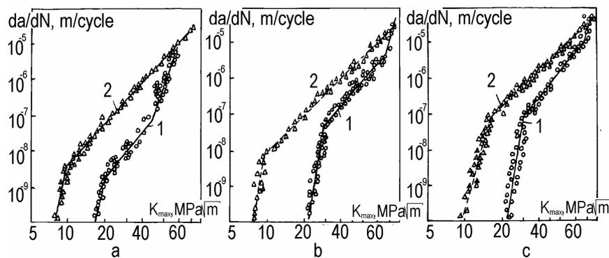
**Figure 6:** FCG diagrams in a weld (1) and in alloy 2V (2) with various content of oxygen in the coordinates “ $da/dN - K_{max}$ ”: a – 0.11% O<sub>2</sub>; b – 0.21% O<sub>2</sub>; c – 0.27% O<sub>2</sub>.
