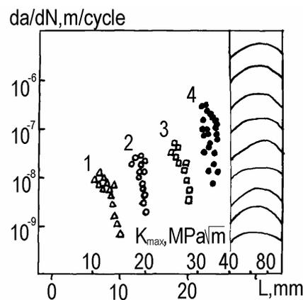
**Figure 5:** FCG diagrams for a welded joint: 1 –  $K_{max} = 12MPa\sqrt{m}$  ;
