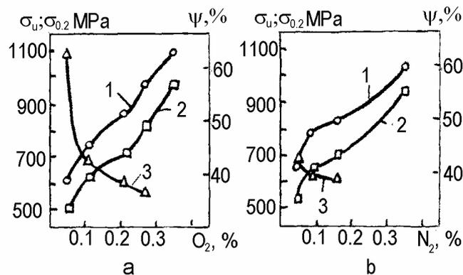
**Figure 1:** The influence of oxygen (a) and nitrogen (b) additives on characteristics of mechanical properties:  $\sigma_u$  (1),  $\sigma_{0.2}$  (2), and  $\psi$  (3) of titanium alloy 2V
