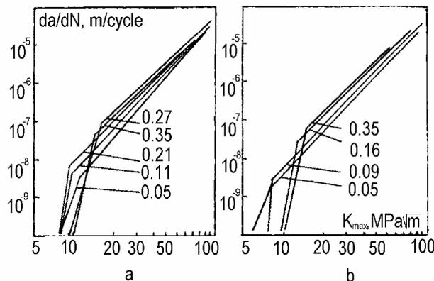
**Figure 3:** Fatigue crack growth (FCG) diagrams for alloy 2V with various contents of oxygen (*a*) and nitrogen (*b*).
