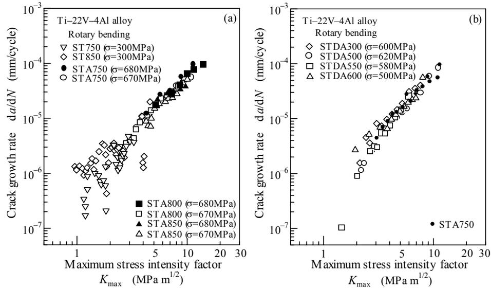
**Figure 3:** Relationships between small crack growth rate and maximum stress intensity factor: (a) ST and STA materials, (b) STDA material.
