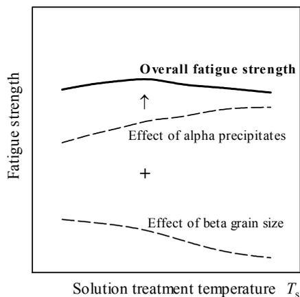
**Figure 5:** Schematic illustration showing effects of grain size and alpha precipitates on fatigue strength in STA materials.
