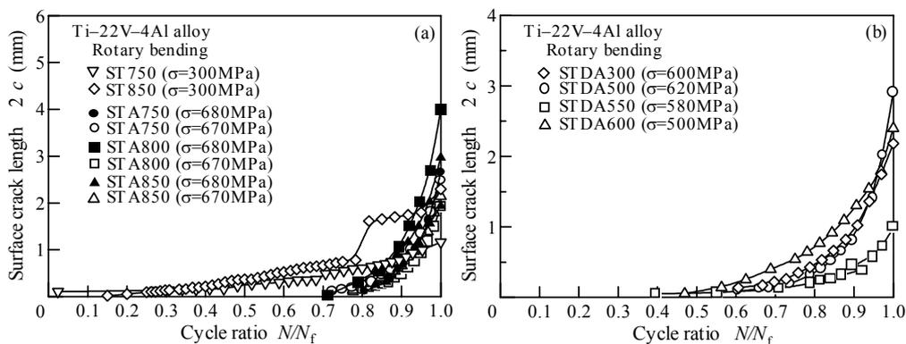
**Figure 2:** Relationships between surface crack length and cycle ratio: (a) ST and STA materials, (b) STDA material.
