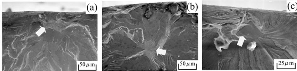
**Figure 4:** SEM micrographs showing subsurface crack origin in STA materials: (a) STA750 ( $\sigma=590\text{MPa}$ ,  $N_f=1.01\times 10^7$ ), (b) STA800 ( $\sigma=640\text{MPa}$ ,  $N_f=7.15\times 10^6$ ), (c) STA850 ( $\sigma=630\text{MPa}$ ,  $N_f=1.63\times 10^7$ ). Arrow indicates the facet.
