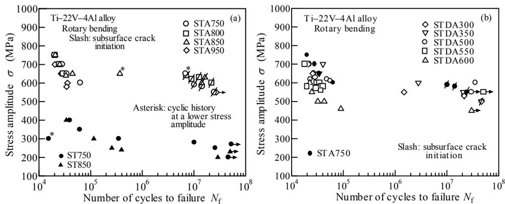
Figure 1:  $S-N$  diagrams: (a) ST and STA materials, (b) STDA material.
