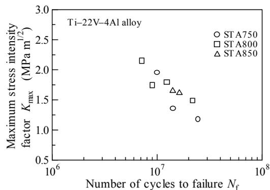
**Figure 6:** Relationship between maximum stress intensity factor for facets and fatigue life.
