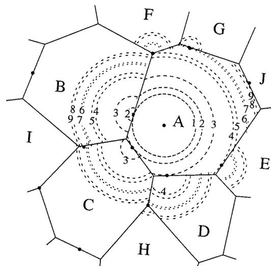
**Figure 1:** Cross-section of a few grains of a model polycrystal. A cleavage crack nucleates in grain A and propagates into neighbouring grains at the sites indicated by dots. The development of the crack is represented by the arcs of circles which are numbered sequentially 1 to 9.
