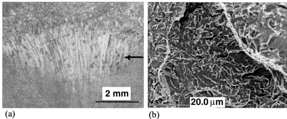
**Figure 4:** (a) Optical micrograph showing the columnar grains in a weld bead; the arrow indicates the fracture path. (b) Scanning electron fractograph of the corresponding fracture surface.
