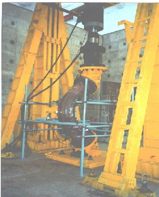
Fig 1: Experimental set up for fatigue and fracture test
