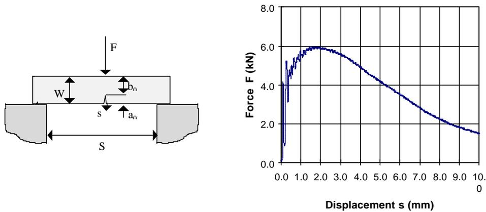
Figure 1 - Mechanical system (left) and the corresponding force-displacement diagram (right) of a bending test with an edge-cracked specimen in the upper-shelf range.
