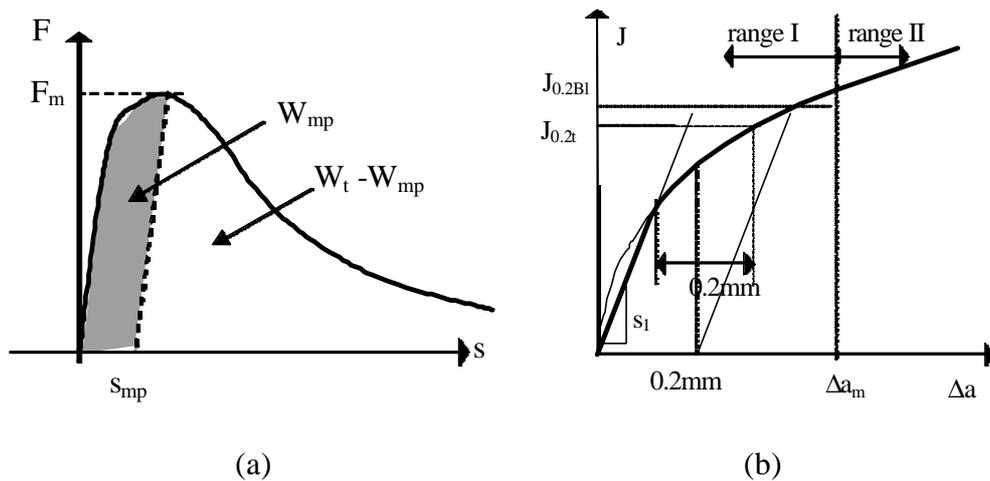
Figure. 2 –Quasistatic force-deflection diagram (a) and calculated J-R-curve (b) of an instrumented Charpy test (schematic)
