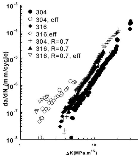
**Figure 3:** Crack Propagation curves  $da/dN$  vs  $\Delta K$  and  $da/dN$  vs  $\Delta K_{eff}$  at room temperature for 316L and 304L
