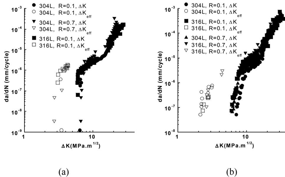
**Figure 8:** Crack Propagation curves  $da/dN$  vs  $\Delta K$  and  $da/dN$  vs  $\Delta K_{eff}$  at 150°C (a) and 300°C (b) on 304L and 316L steel
