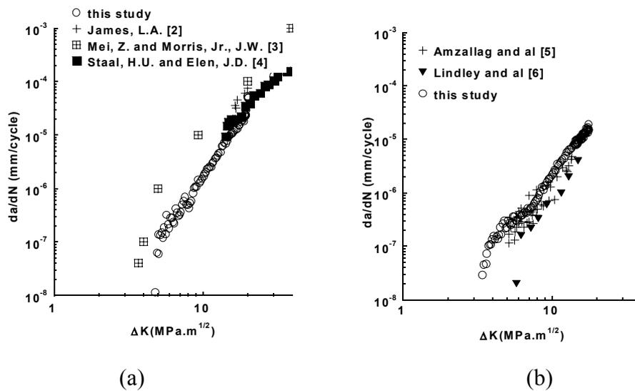
**Figure 2:** Crack Propagation curves  $da/dN$  vs  $\Delta K$  at room temperature for 304L (a) and 316L (b) steels.
