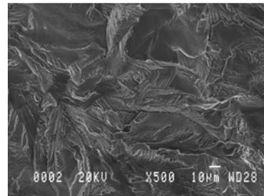
**Figure 4:** Fracture surface morphology in the near-threshold range.
