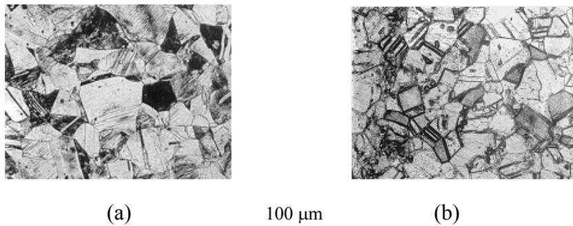
**Figure 1:** Microstructure of 304L (a) and 316L (b) alloys
