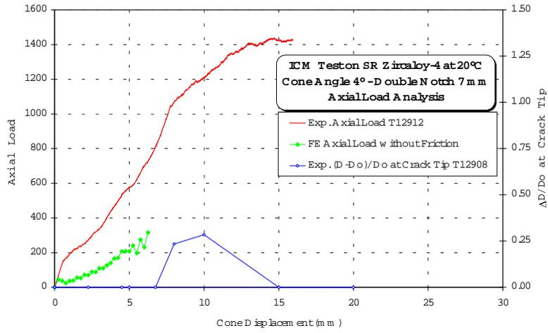
Figure 5 : Loading Diagram for an ICM test at room temperature.
