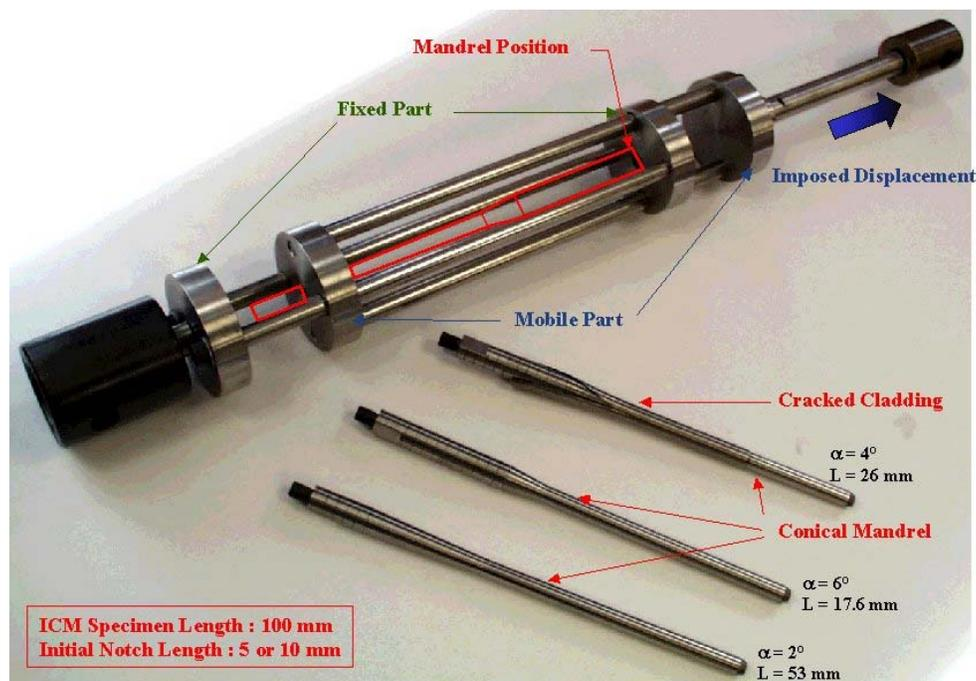
Figure 1 : ICM Testing Device.
