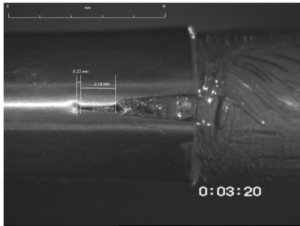
Figure 2 : View of ICM Test T12912 for  $\Delta a = 0.22$  mm.
