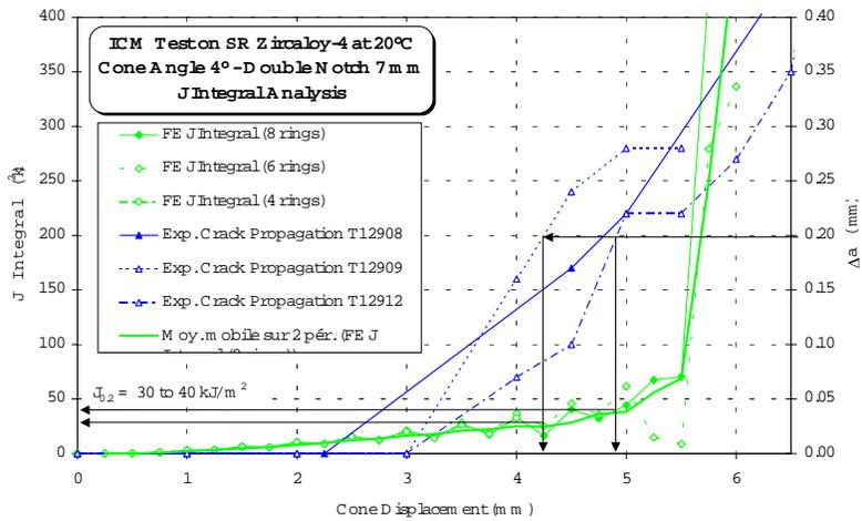
Figure 7 : Determination of J integral for a crack propagation of 0.2 mm.
