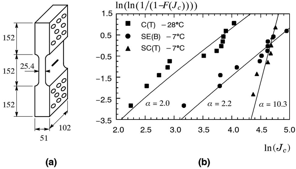
**Figure 1** (a) Geometry of bolt-loaded surface crack specimen; (b) Weibull plots of experimental toughness values at  $T = -28^\circ\text{C}$  and  $-7^\circ\text{C}$  [7].
