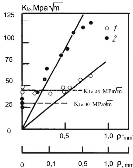
Fig. 8. Dependence between fracture toughness  $K_{Ic}(\rho)$  and acuity  $\rho$ : 1 - grain size 300  $\mu\text{m}$ ; 2 - 28  $\mu\text{m}$ .
