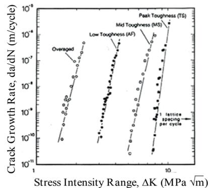
Fig. 6. The subcritical crack growth relations for ceramics [12].
