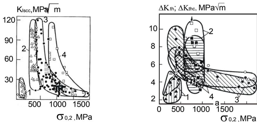
Fig. 4. LAD's for various materials tested in 3% water solution of NaCl: 1-aluminium alloys; 2-titanium alloys; 3-low alloyed steels; 4-stainless steels.
