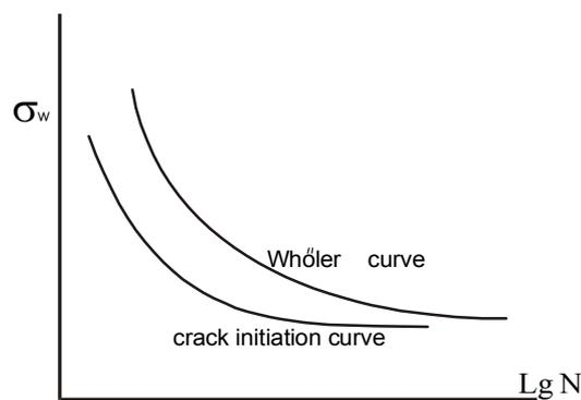
**Fig. 2.** Wöhler and crack initiation curves for typical low and middle strength alloys.
