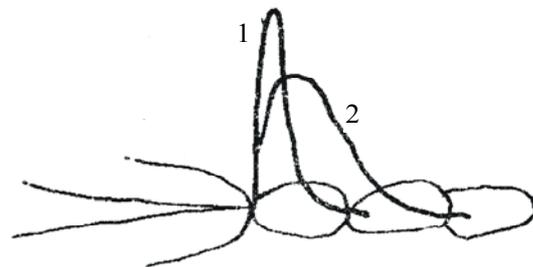
**Fig. 10.** Process zone size as a function of the notch acuity ( $l$ ,  $2$ ). For short process zone size the instant rupture can occur inside the critical cell of embrittlement (curve  $1$ ).
