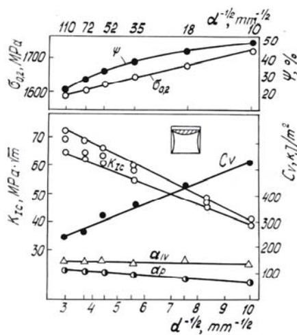
Fig. 7. Variation of the mechanical properties of 0.4C-1Cr (40Ch) steel with prior austenite grain size,  $d$ .
