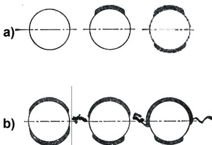
**Fig. 9.** Damaging stages near the critical constellation of particles: a) initial debonding; b) linking deterioration.
