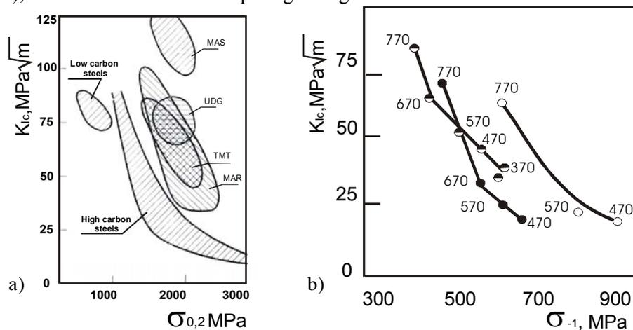
**Fig. 1.** a) LAD ( $K_{Ic}-\sigma_{0.2}$ ) for structural steels: MAR — maraging steels, TMT — thermo-mechanical treatment; UDG — ultra dispersion grains; MAS — metastable austenitic steels. b) LAD ( $K_{Ic}-\sigma_{-1}$ ) for various chromium steels (ShCh15, 7Ch3, 40Ch). Figures near the points determine the tempering temperature ( $^{\circ}\text{K}$ ) after quenching.
