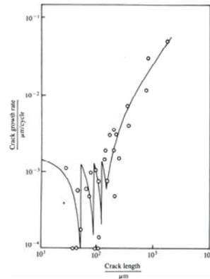
**Fig. 3.** Crack growth kinetics in the region of short crack propagation.
