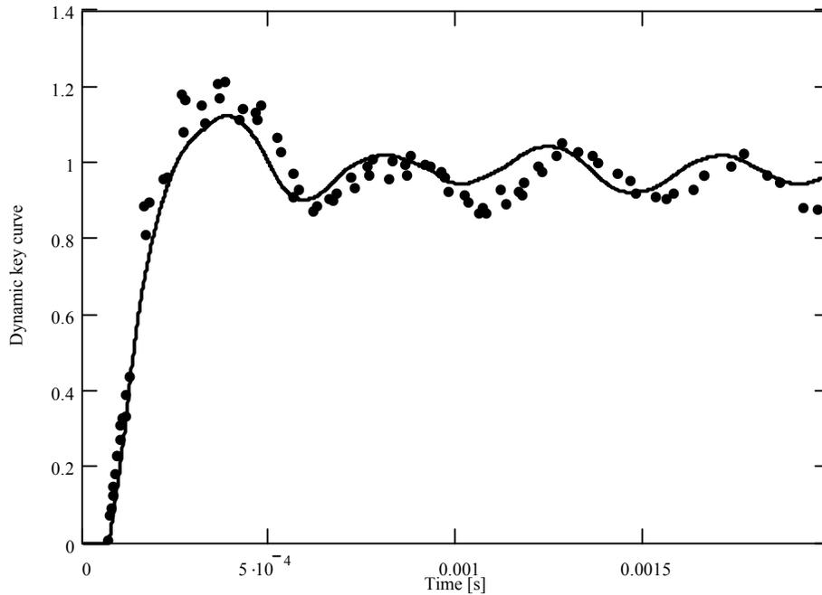
Figure 2: Comparison of the numerical dynamic correction function for steel striker and steel anvil with measurements from [7]
