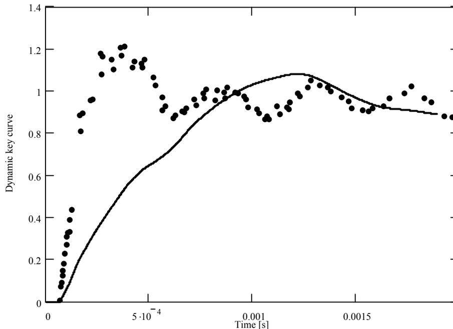
**Figure 3:** Comparison of the numerical dynamic correction function for PE striker and steel anvil with measurements from [7]
