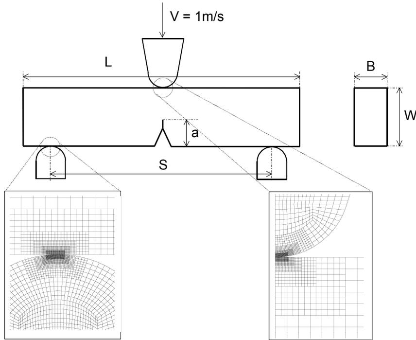
**Figure 1:** Specimen configuration and mesh refinement
