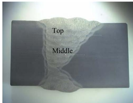
**Figure 1:** Typical macro section of the welded joints
