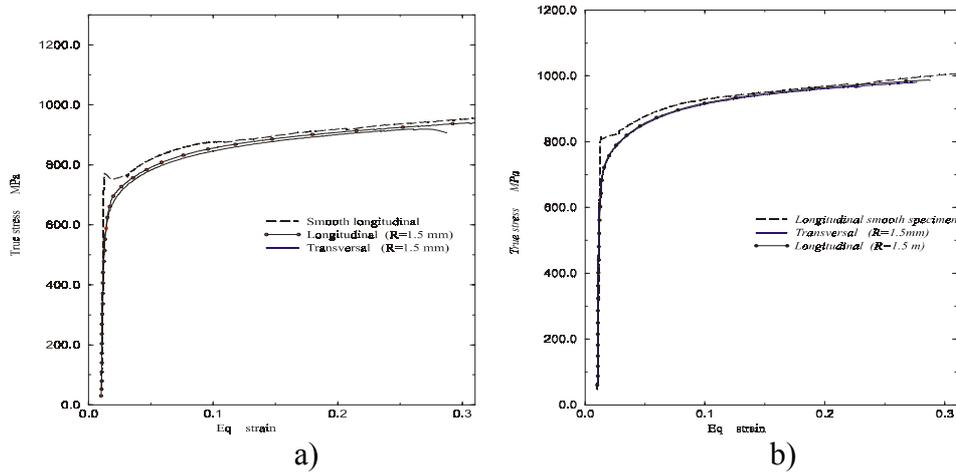
**Figure 4:** True stress strain curves derived from notch tensile results
