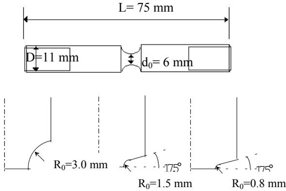
**Figure 2:** Notch tensile specimen dimensions
