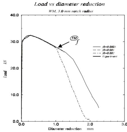
Figure 5: Fitting of initial void volume fraction,  $f_0$
