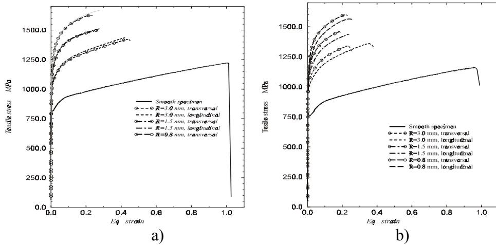
**Figure 3:** Tensile stress strain curves from notch tensile testing of
