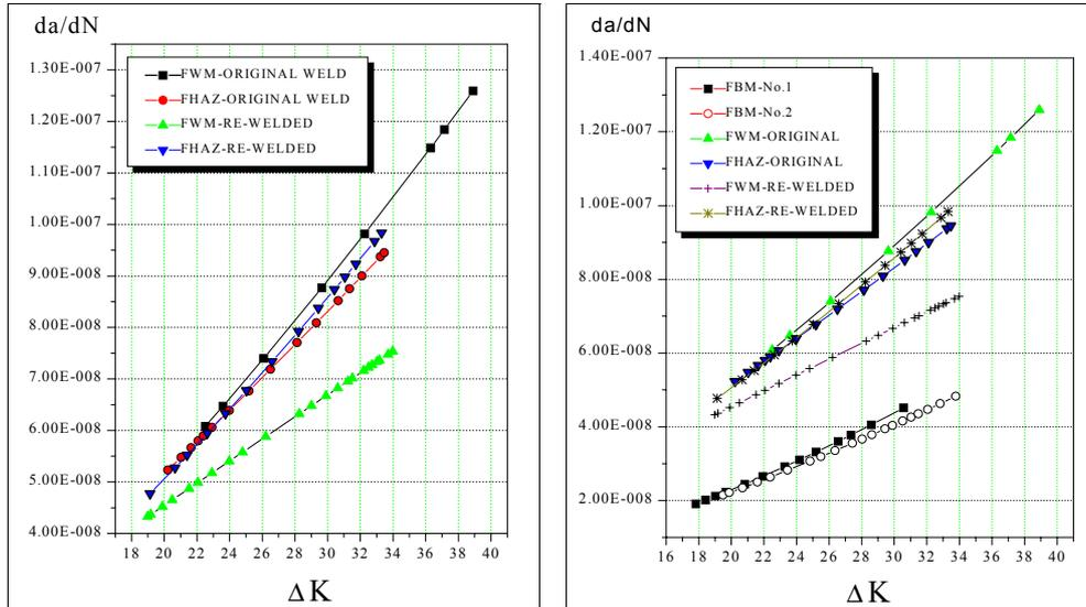
Figure 4:  $da \times dN$  curves from all the mentioned conditions.
