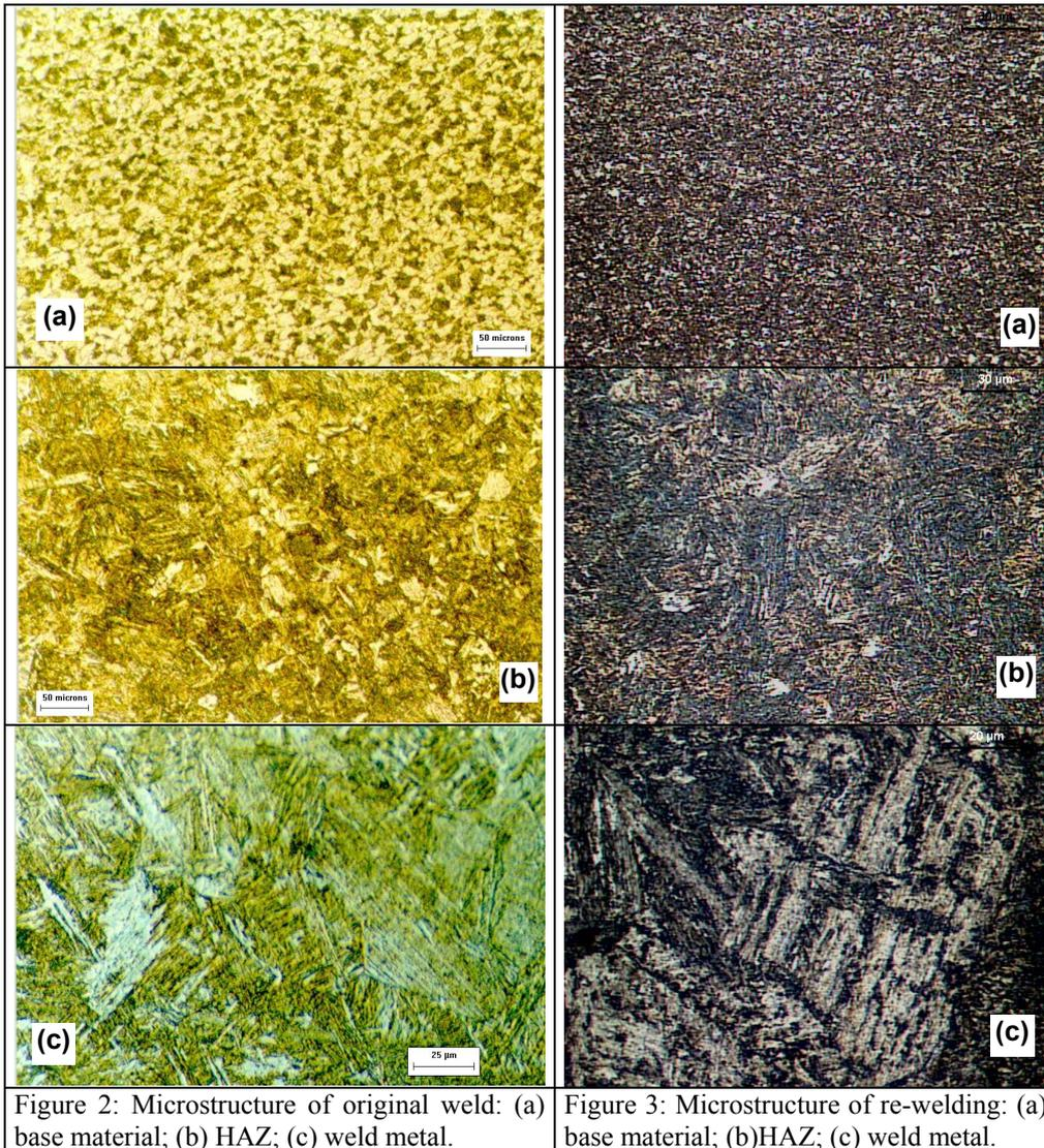
From Figure 2(a), one can see that the base material contains a microstructure of fine grains, formed by ferrite and perlite. So, the fatigue crack will find larger resistance to propagate through the ferrite and perlite grains due to the microstructural barriers offered. From Figure 2 (c), it is
