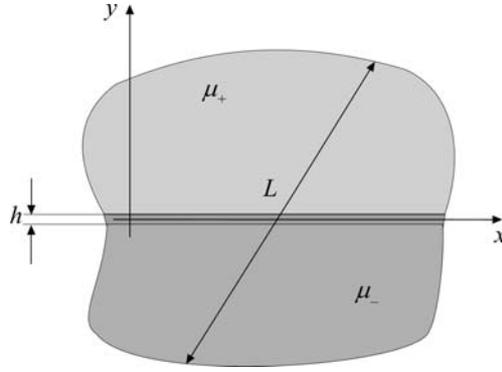
Figure 1. Bimaterial solid with thin stiff interface
