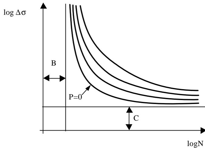
**Figure 1** - S-N field with percentiles curves in the fatigue model of Castillo et al. [1,3].
