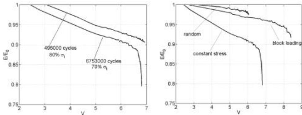
**Figure 4.** Stiffness curves of the IM7/8552  $[0/90]_{4s}$  laminate in function of  $V$  a) for constant stress fatigue and b) for different fatigue load histories.
