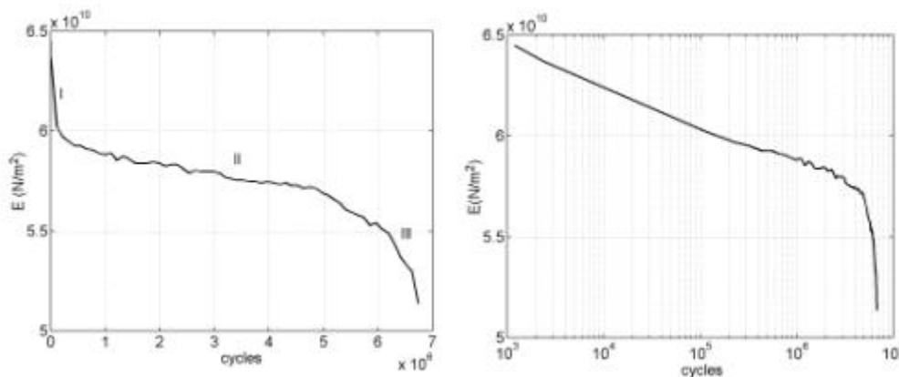
**Figure 3.** Stiffness curves for constant stress and low load levels
