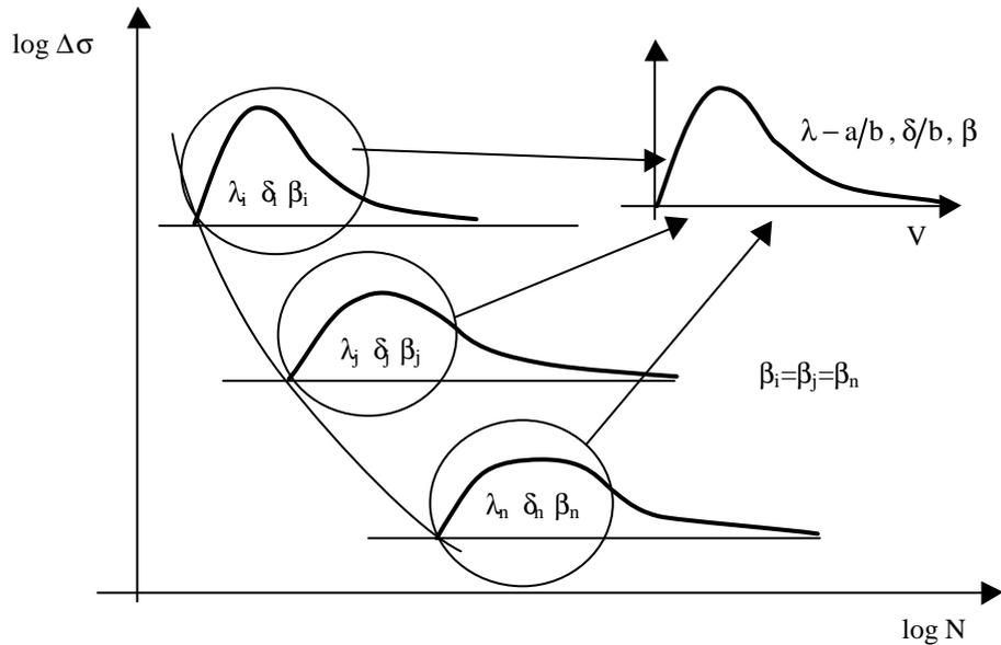
**Figure 2** - S-N field with pdfs of log N at different stress ranges and corresponding pdf of the normalized lifetime, V.
