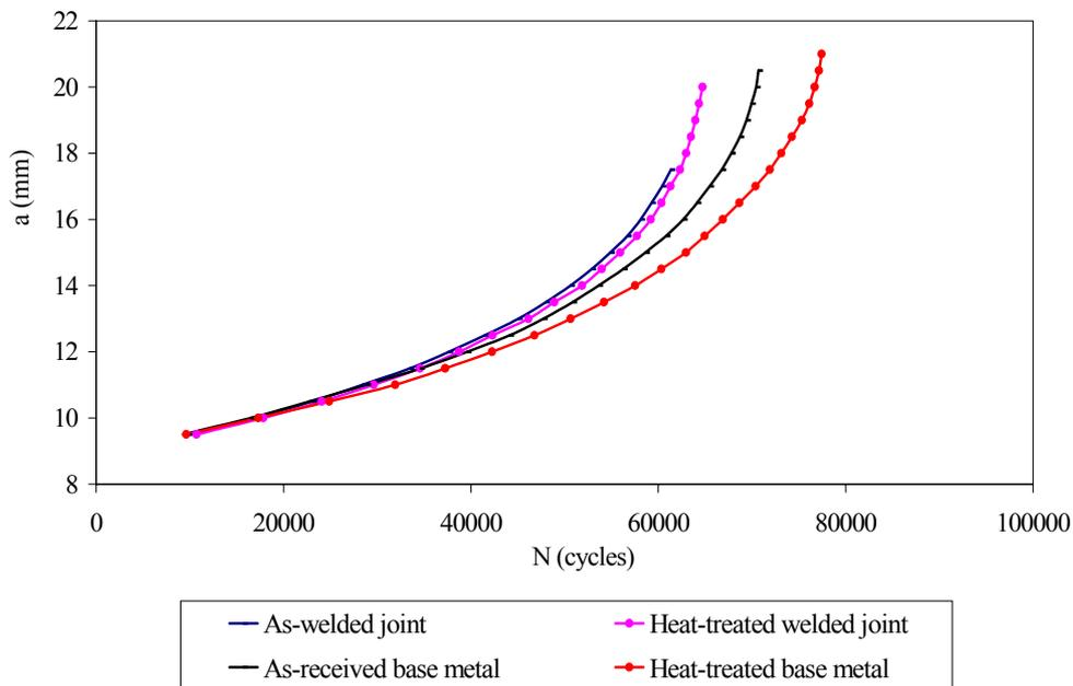
**Figure 1:** Variation of crack length ( $a$ ) with the number of cycles ( $N$ ) under constant amplitude loading.
