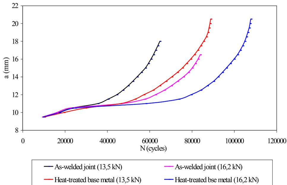
**Figure 3:** Effect of single overloads of 13.5 and 16.2 kN on the a-N curves.
