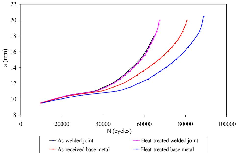
**Figure 2:** Variation of crack length (a) with the number of cycles (N) for a single overload of 13.5 kN.
