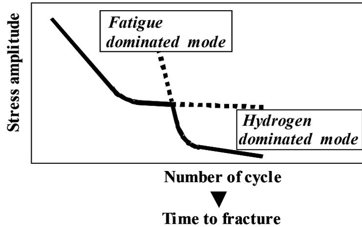
**Fig.3. Two modes of fatigue crack development in hydrogen environment.**
