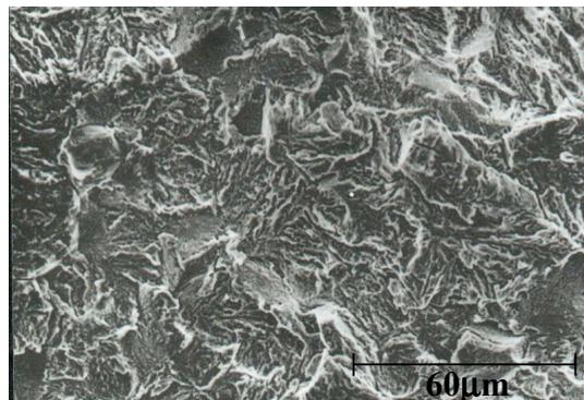
**Fig.4. SEM photograph of QC facet on the specimen at 150MPa,  $N_f=168,420$ .**
