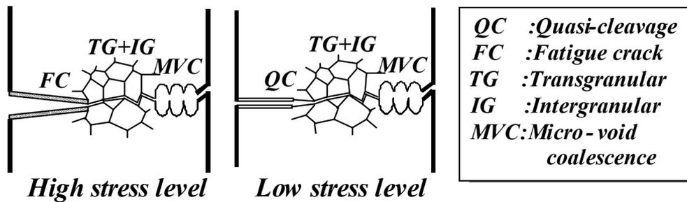
**Fig.6. Models of fatigue crack development in hydrogen environment.**
