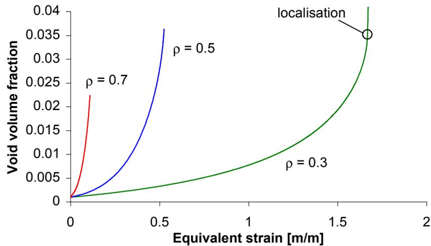
**Figure 4:** Void volume fraction for monotonic loading.
