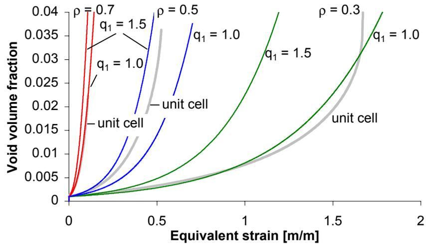
**Figure 6:** Comparison of the GTN damage and fraction model with the unit cell for monotonic loading.
