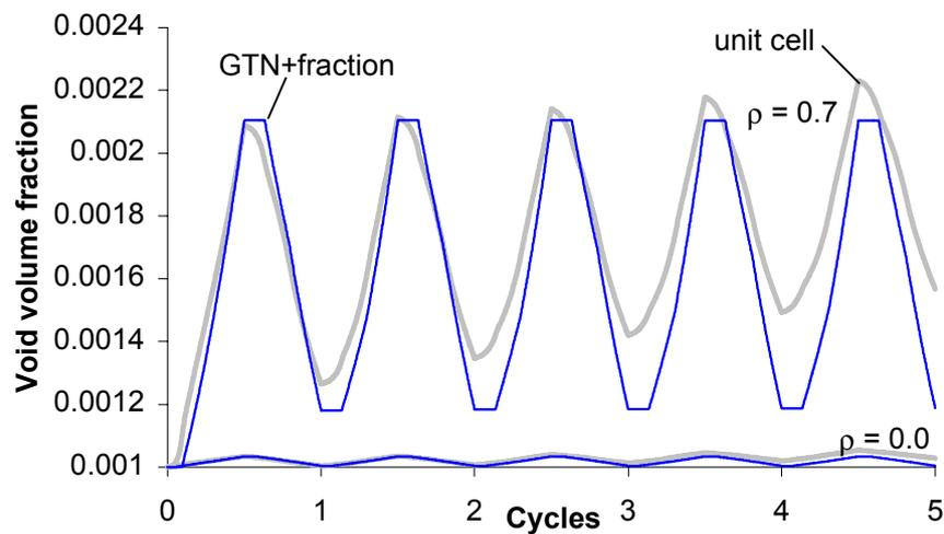
**Figure 7:** Comparison of the combined GTN damage and fraction model with the unit cell calculations for cyclic loading.
