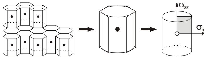
**Figure 3:** Micromechanical modelling of a material containing voids.
