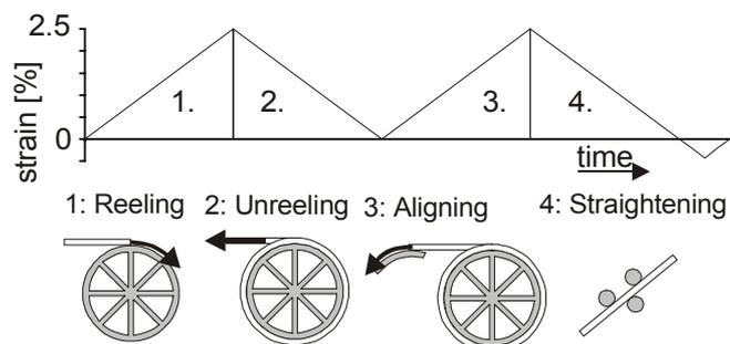
**Figure 1:** The reeling process and the corresponding deformations.
