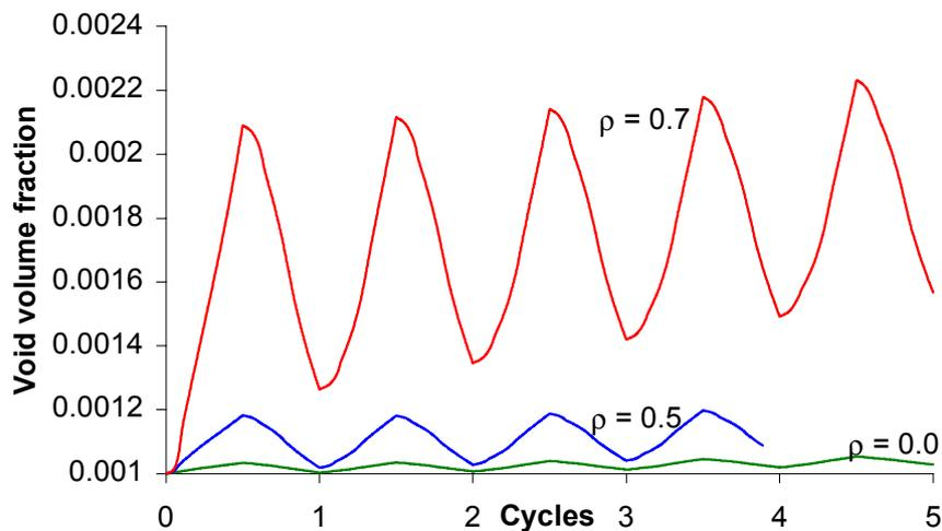
**Figure 5:** Evolution of the void volume fraction during cyclic loading for different triaxialities.
