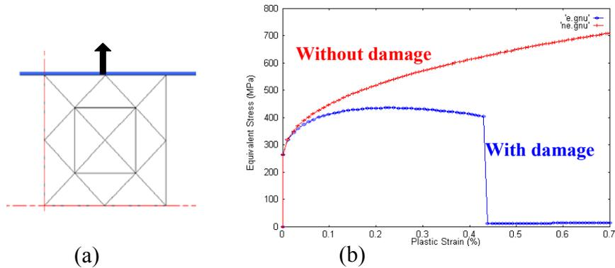
**Figure 3:** Uniaxial tensile test with coupled damage
