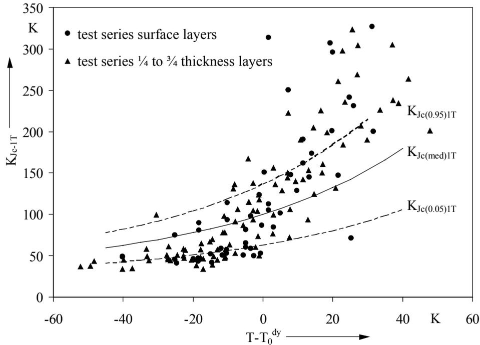
Fig. 1 Thickness corrected dynamic fracture toughness  $K_{Jc-1T}$  for material investigated
