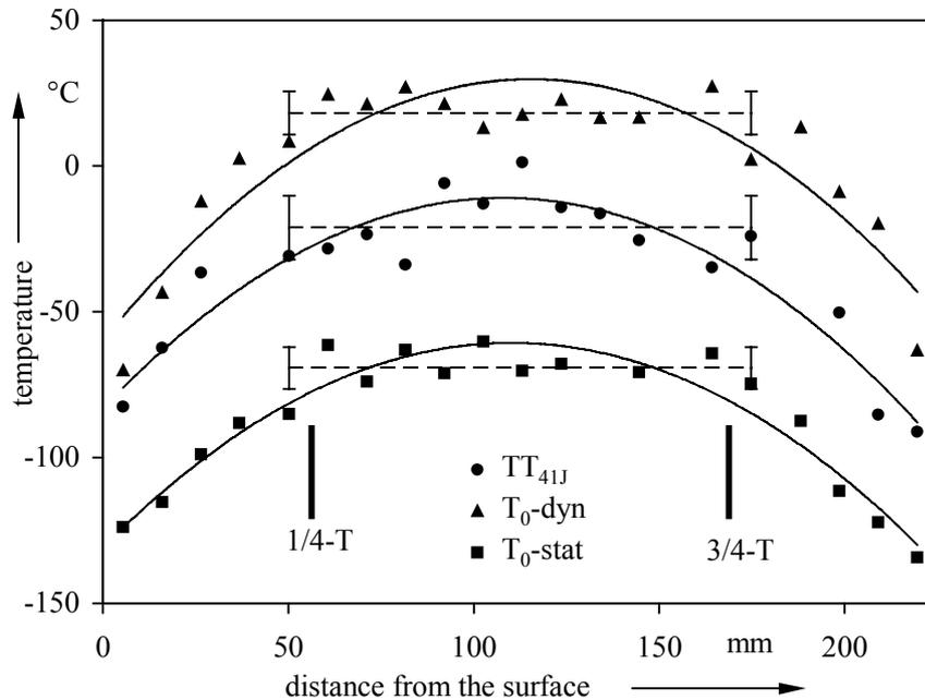
Fig. 2 Effect of specimen location on the ductile-brittle transition temperature determined by dynamic ( $T_0^{\text{dyn}}$ ) and static ( $T_0^{\text{stat}}$ ) master curve procedure and Charpy-V impact tests ( $TT_{41J}$ )
