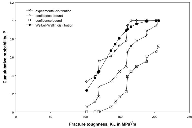
Fig. 4 Comparison of the experimental distribution and the Weibull-Wallin distribution for  $T_{\text{Test}} = 16,9$  °C, dynamic loading
