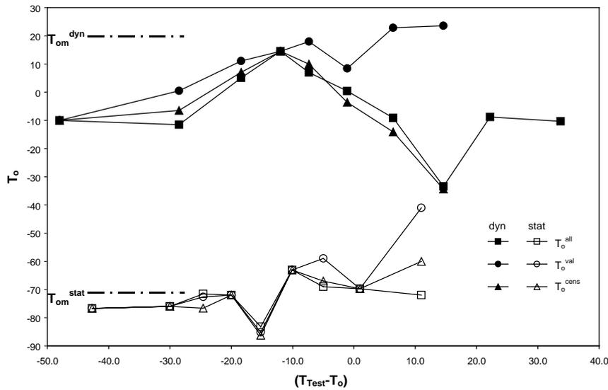
Fig. 3 Effect of the test temperature on  $T_0$  under static ( $T_0^{\text{stat}}$ ) or dynamic ( $T_0^{\text{dyn}}$ ) loading using all values measured ( $T_0^{\text{all}}$ ), valid values ( $T_0^{\text{val}}$ ) or valid and censored values ( $T_0^{\text{cens}}$ )
