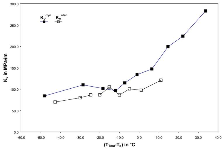
Fig. 5 Temperature dependence of the Weibull distribution normalization fracture toughness,  $K_0$  for dynamic and static loading
