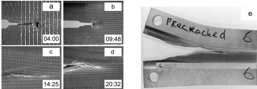
**Figure 3:** showing a)-d) four captured frames showing crack propagation in 4mm thick ligament specimen No. 6. Time from the start of the test is shown in the right bottom corner in format `minutes:seconds`; e) 4mm thick shear specimen after the test.
