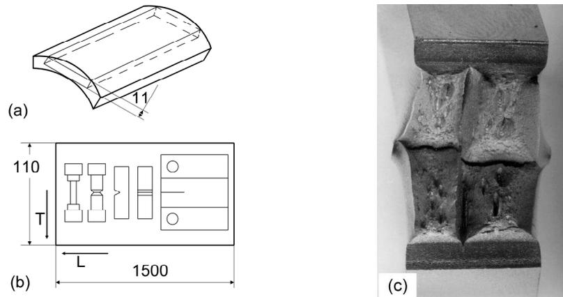
**Figure 1:** showing a) orientation of a plate of material cut out of a pipe, b) orientation and position of specimens machined and c) Fracture surface of a Charpy specimen machined of X80 grade API L5 pipeline showing areas of initial flat fracture, shear lips, delaminations and the region of final shear fracture.
