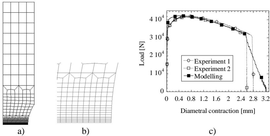
**Figure 2:** showing a) axisymmetric finite element mesh of a quarter of a notch tensile specimen with notch radius  $r = 6$  mm, b) enlarged bottom area of the mesh, c) experimental and best-fitted modelling 'load – diametrical contraction' curves for specimens with  $r = 6$  mm.
