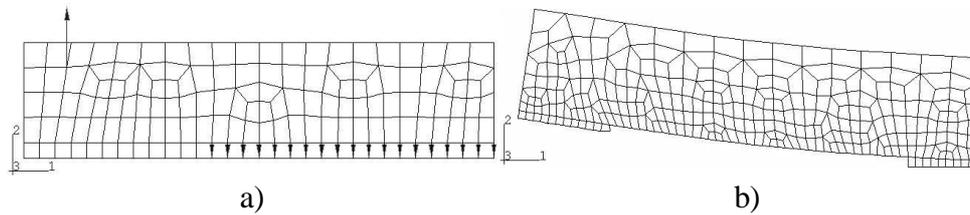
**Figure 5:** showing a) initial and deformed meshes of half of an 8-mm thick ligament shear specimen.
