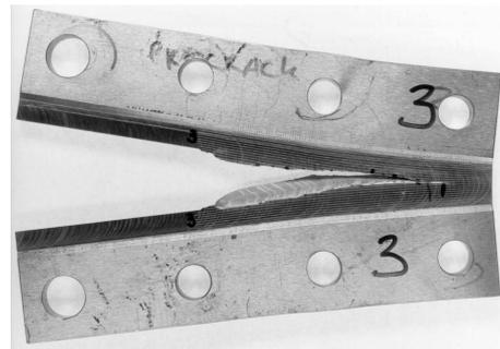
**Figure 4:** showing a) CTOA as a function of crack growth and b) 8mm thick shear specimen after the test.
