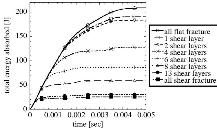
**Figure 6:** Charpy energy – time curves for different amounts of shear layers obtained via FE modelling.
