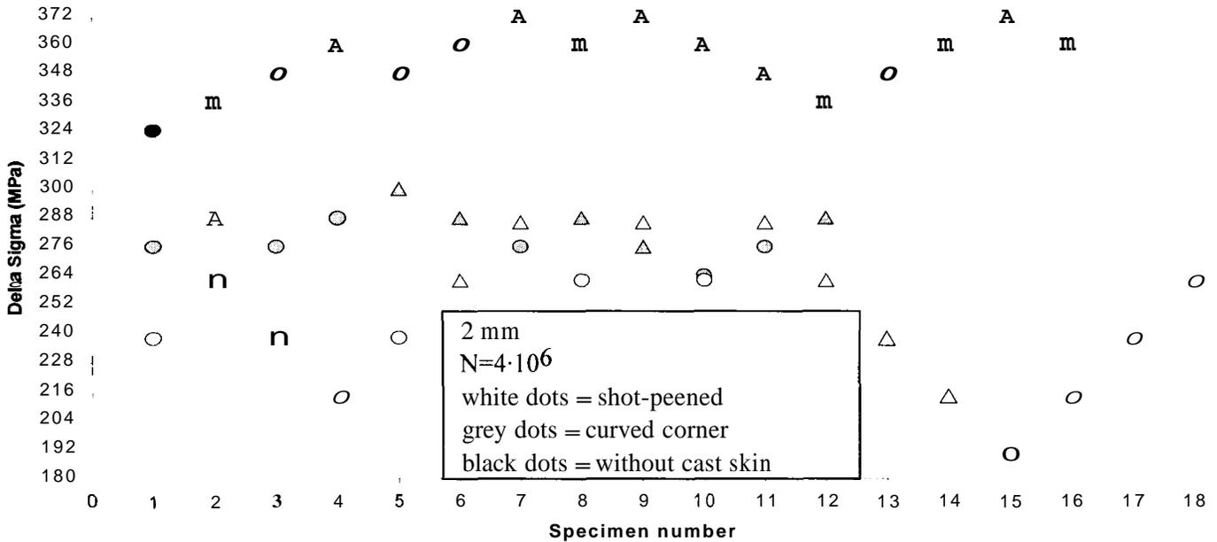
Figure 3: Staircase results of the 2 mm specimens, R=0.1.
