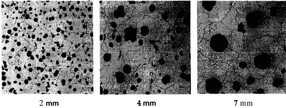
**Figure 1:** Metallographic structures of the investigated nodular cast iron (marker = 20  $\mu\text{m}$ ).
