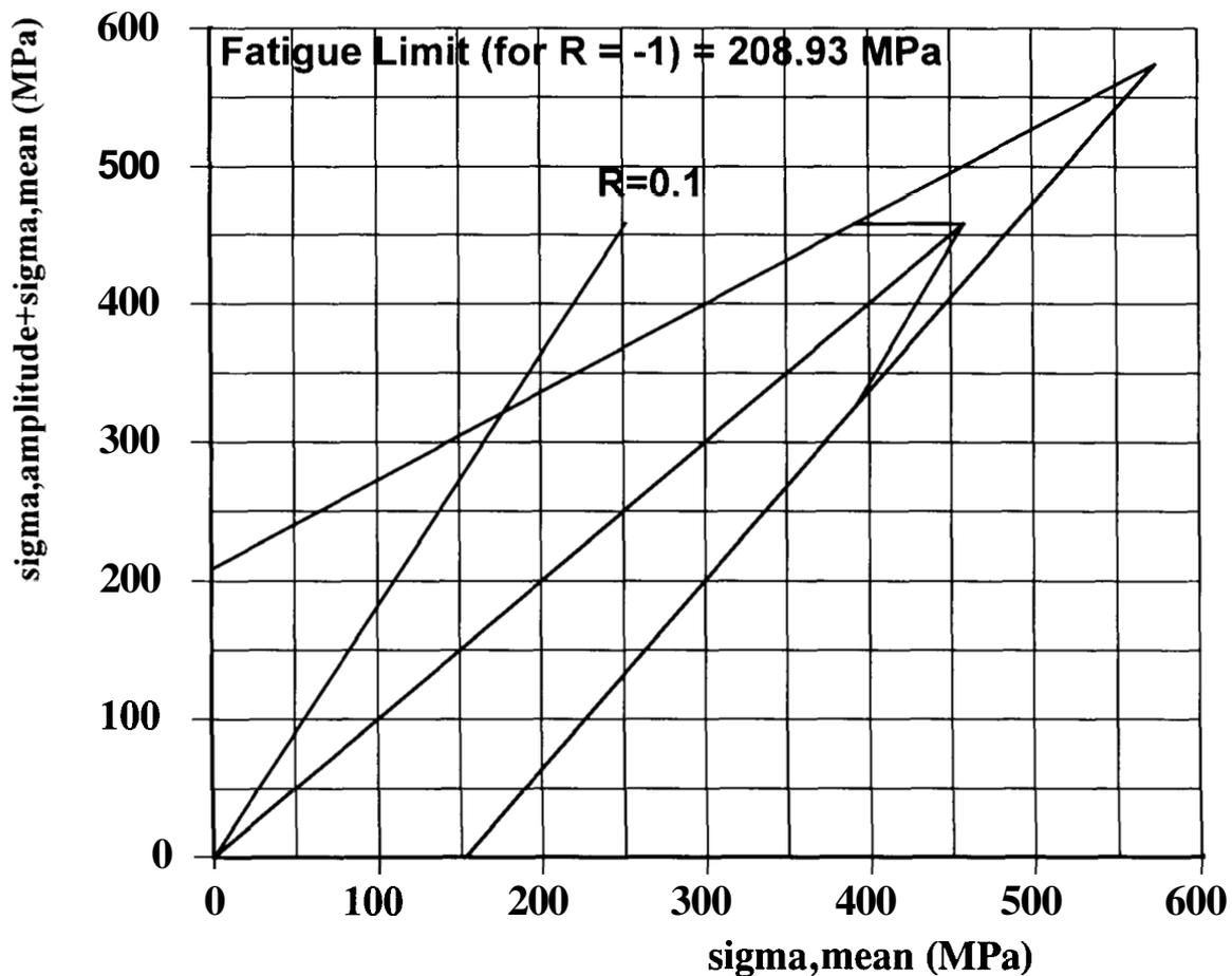
**Figure 5:** Smith diagram of 2 mm thick cast iron specimens with cast skin and curved corners, the line for  $R=0.1$  is shown.
