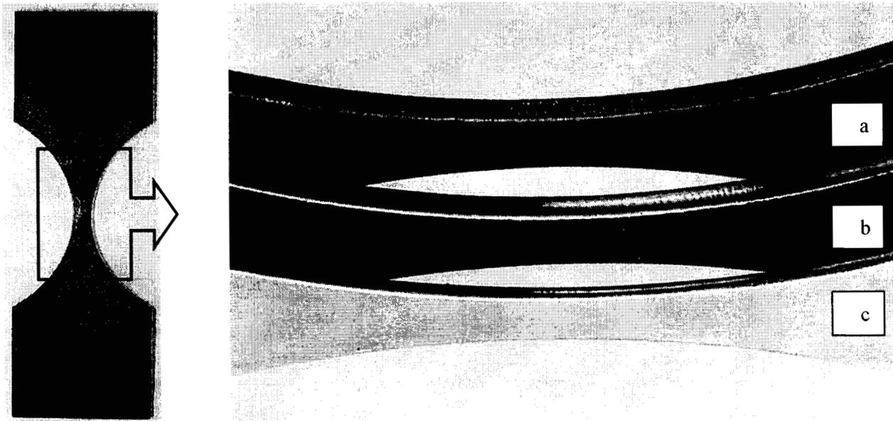
**Figure 2:** Different surface geometry's of the 2 mm tensile specimens (a: cast skin and shot-peened, b: cast skin and curved corners and c: without cast skin and with curved corners).
