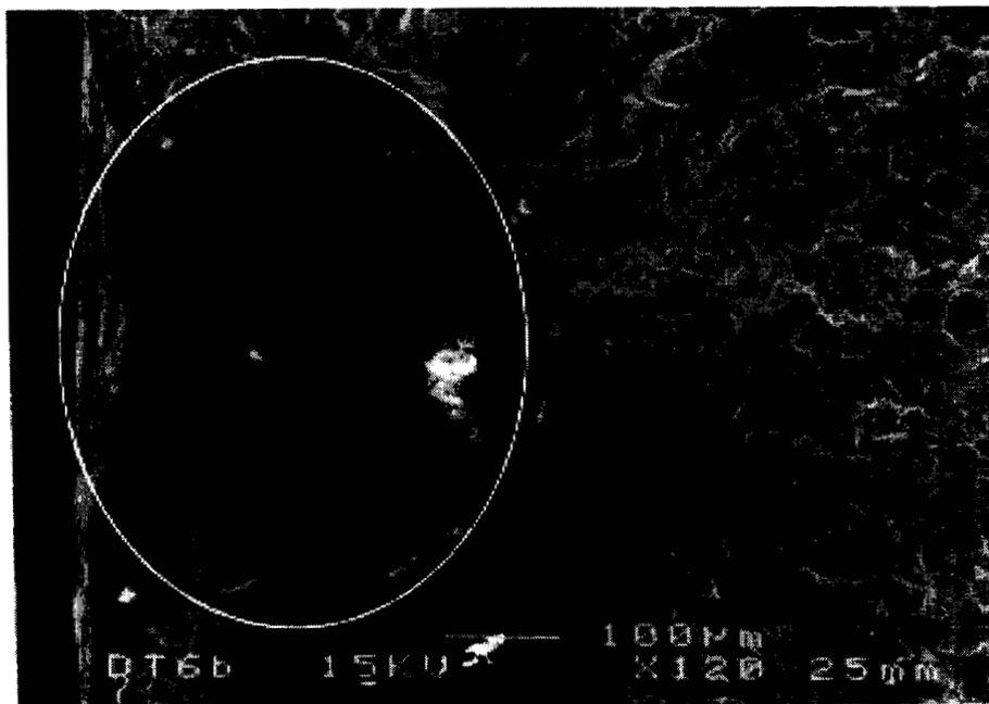
Figure 6: Initiation area of crack growth near the cast skin of a 4 mm specimen.
