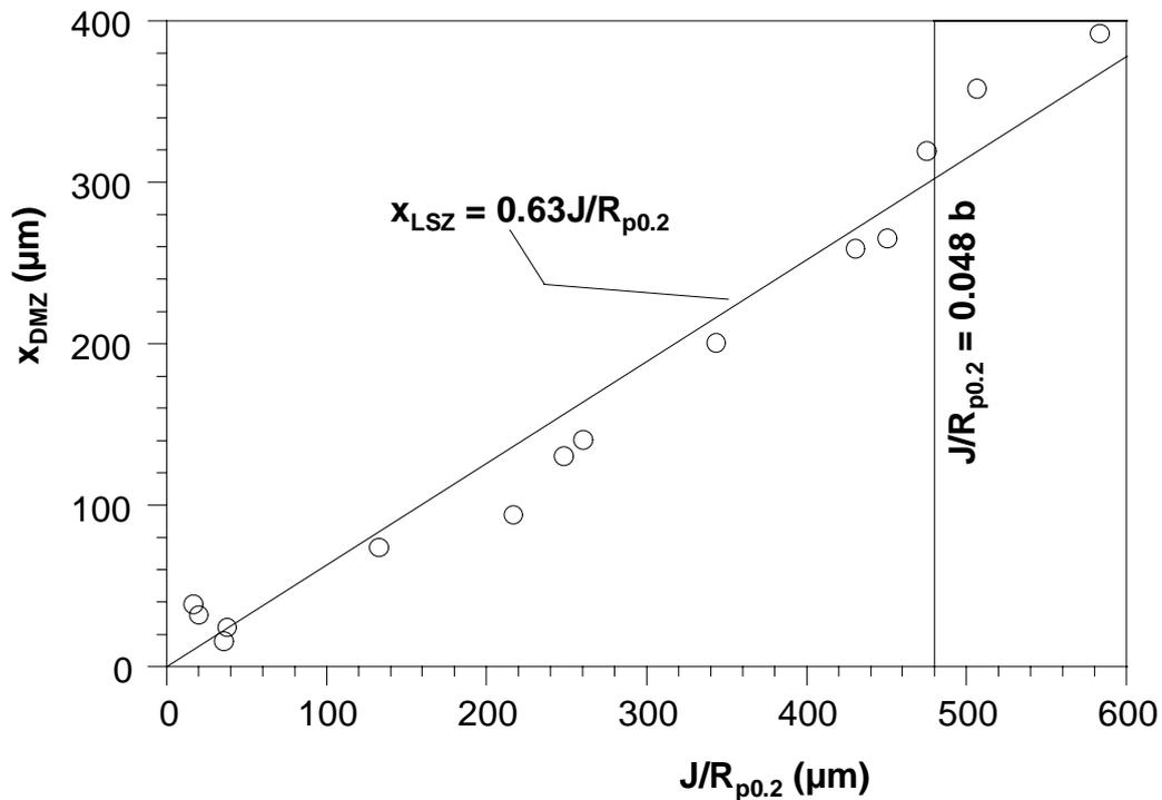
**Figure 5:** Comparison of the measured length of the ductile morphology zone ( $x_{DMZ}$ ) and the theoretical length of the large strain zone ( $x_{LSZ}$ ).
