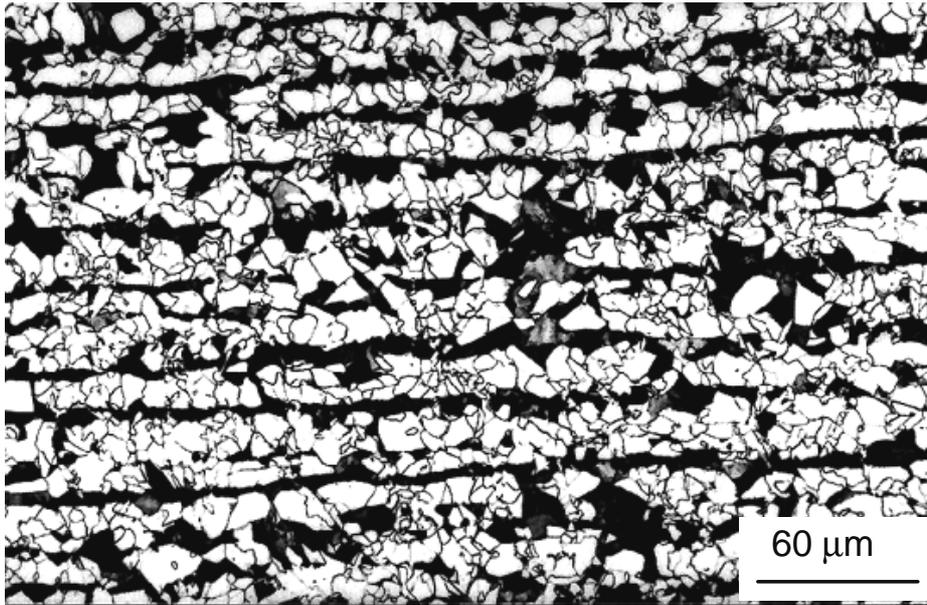
**Figure 1:** Ferritic-pearlitic microstructure of the investigated low carbon steel
