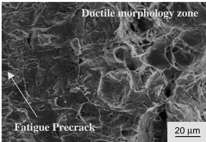
**Figure 3:** The fatigue precrack (at the left) and the ductile morphology zones (at the right).
