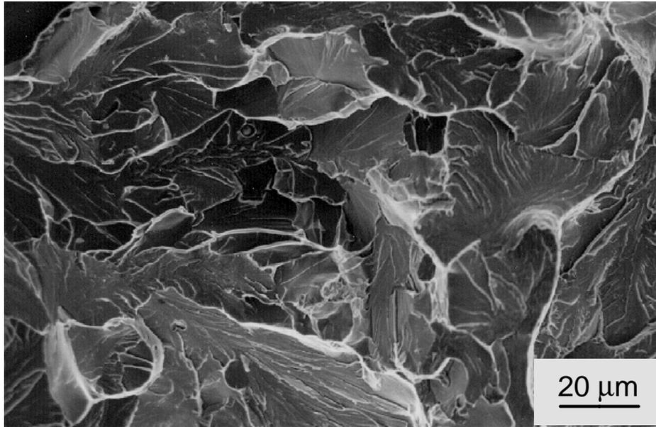
**Figure 4:** The final fracture zone showing a typical cleavage pattern
