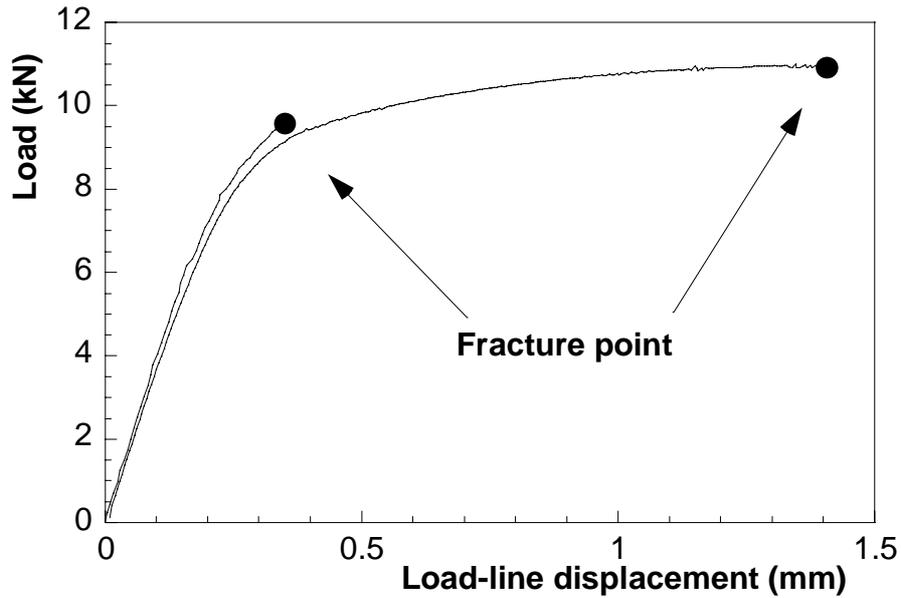
**Figure 2:** Load versus load-line displacement curves obtained in two fracture tests.
