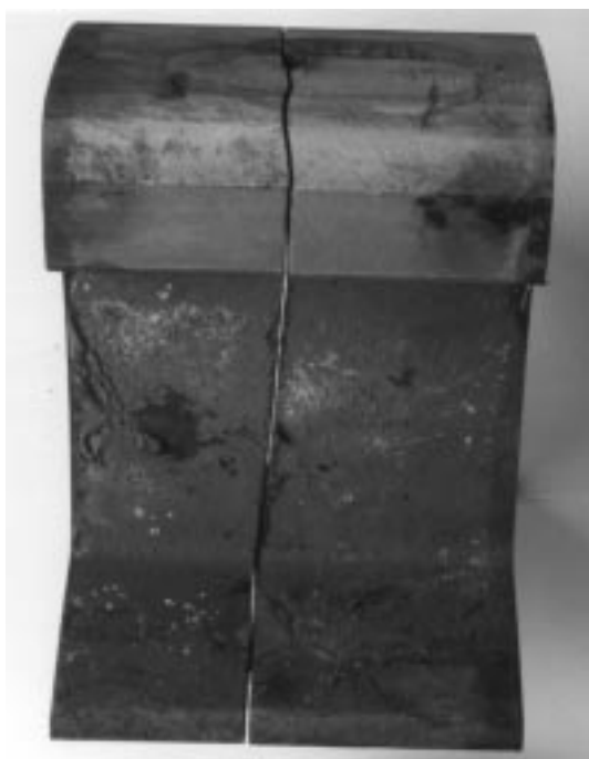
Figure 3: Fracture of a HSH Rail (Head Special Hardened)
