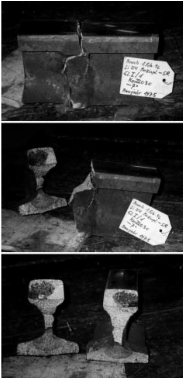
Figure 5: Example 2; Wheel-Slip Mark
