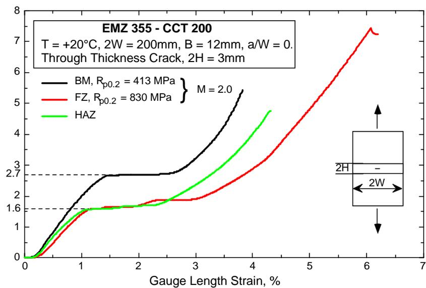
Fig. 4 Stress-Strain, CTOD-Stress and crack driving force diagrams of the 355 MPa steel
