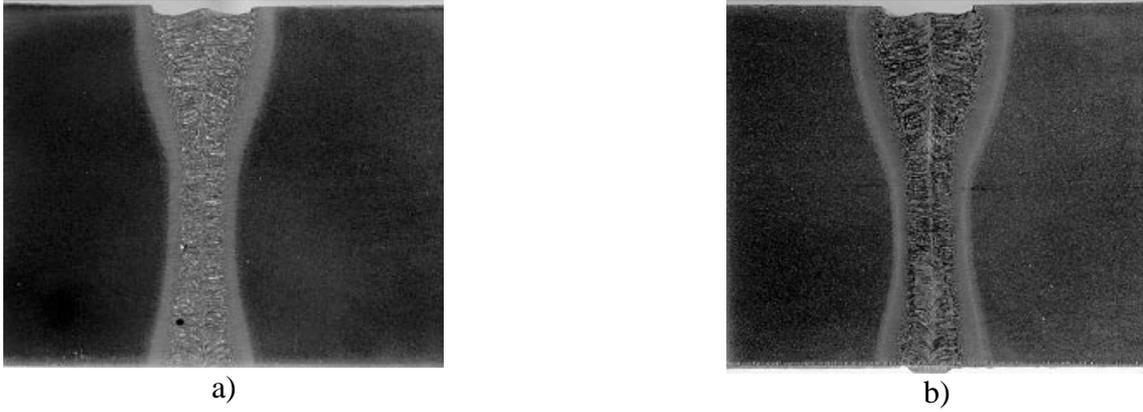
Fig. 1. Macrographs of 12 mm thick 17kW CO<sub>2</sub> laser welded steel plates;
