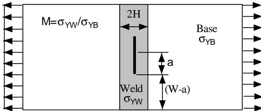
Fig. 2 Schematic showing the dimensions of the laser welded center cracked wide plate:
