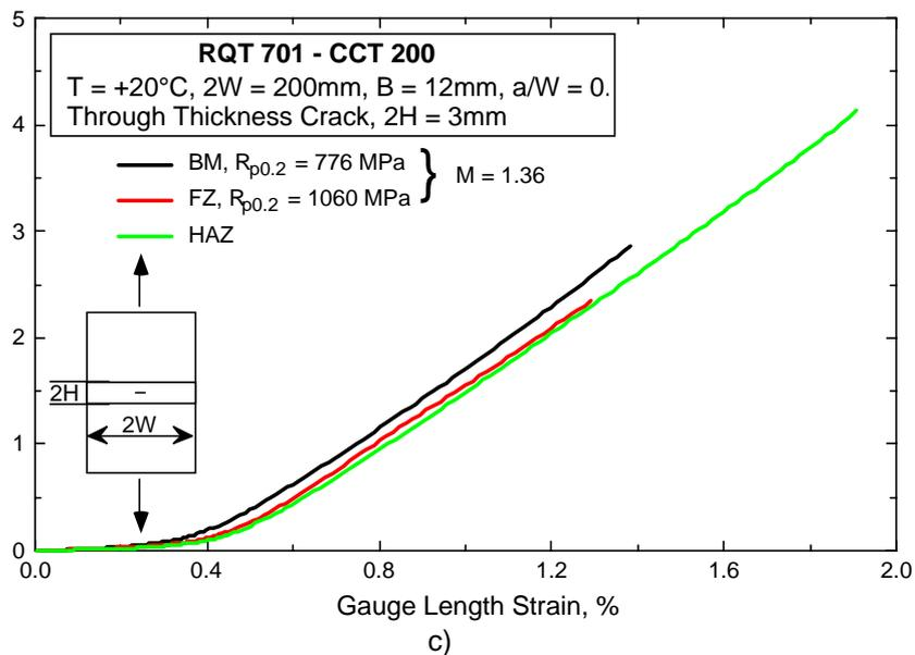
Fig. 5 Stress-Strain, CTOD-Stress and crack driving force diagrams of the 701 MPa steel
