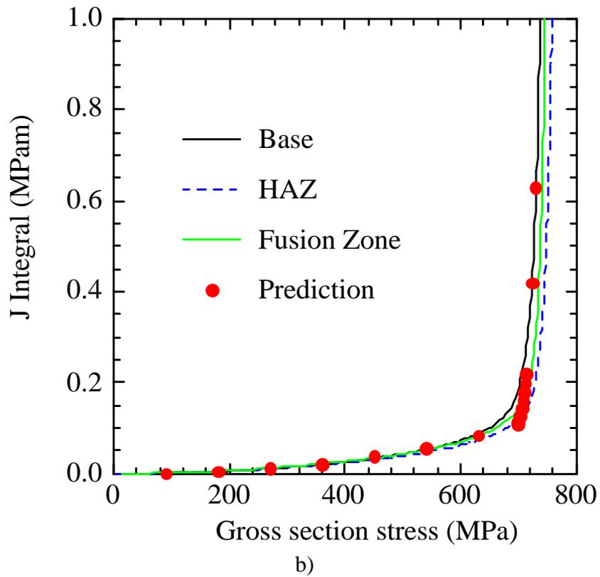
Fig. 6 Comparison of the experimental wide plate results and SINTAP procedure predictions for;
