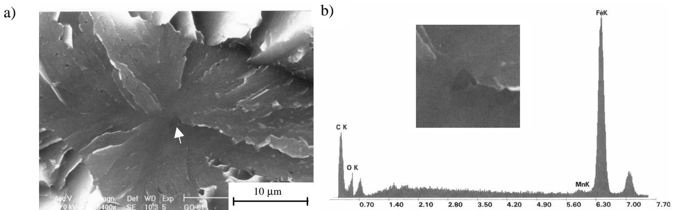
**Figure 2:** a) Fractograph of a broken 4PB specimen, showing a carbide in the fracture initiation. b) EDS analysis of the fracture triggering feature.
