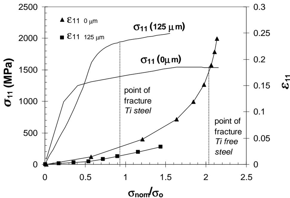
**Figure 5:** Evolution of  $s_{11}$  and  $e_{11}$  in the fracture initiation site in a TiN containing steel (brittle zone cracking initiated cleavage) and in similar Ti free steel (microvoid driven cleavage initiation).
