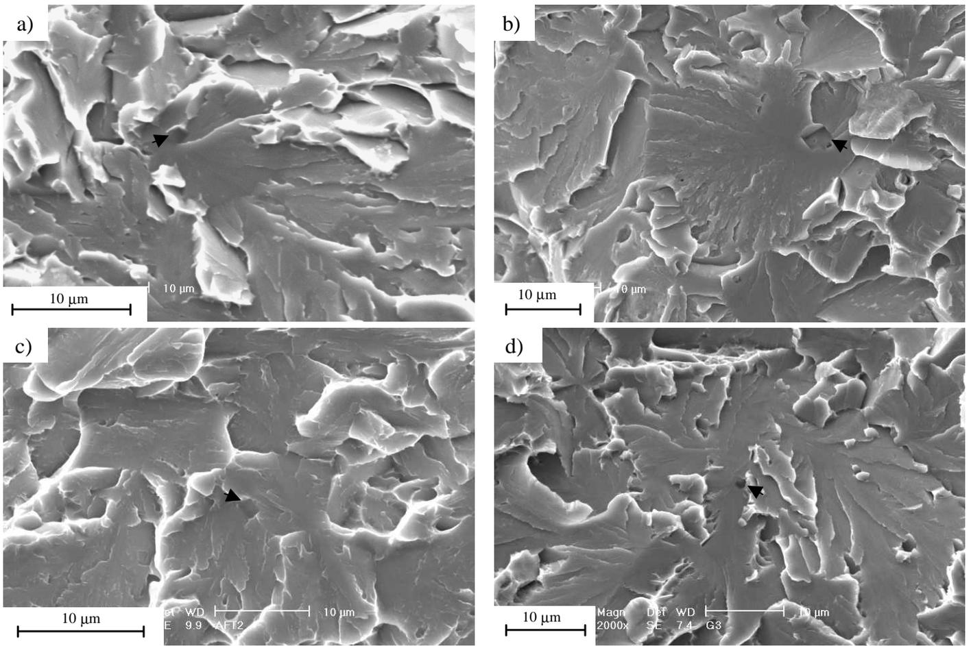
**Figure 1:** Broken TiN particle in the main origin of fracture in a four point-bending specimen in a) bainite, b) ferrite+pearlite, c) martensite and d) bainite.
