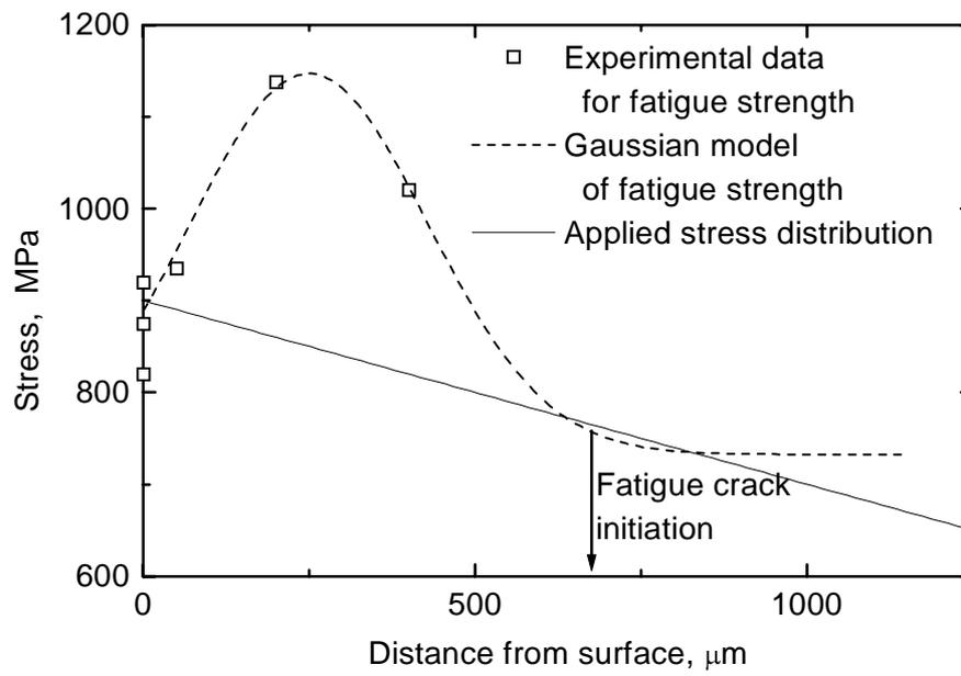
Fig. 5 Gaussian model of fatigue strength variation with distance from surface.
