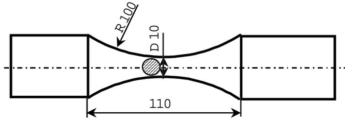
Fig. 1a. Specimen geometry for fatigue testing.
