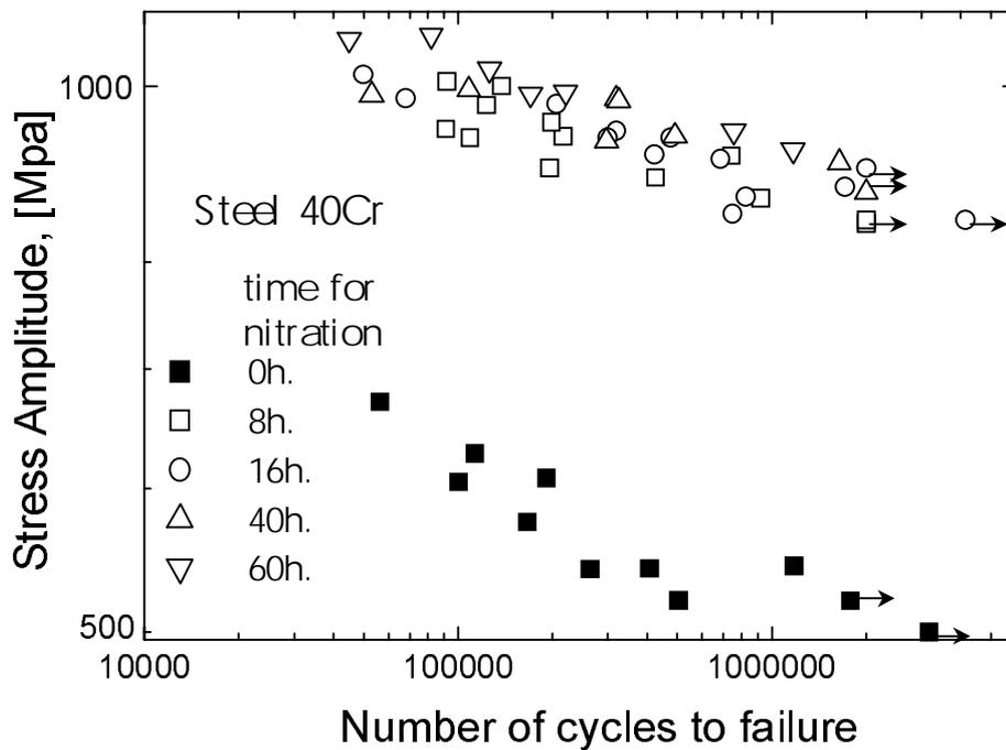
Fig. 2. S-N curves for steel 40Cr annealed specimens and after ion nitration.
