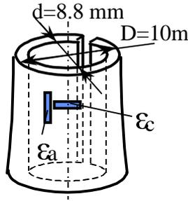
Fig1b. Specimen dimensions after residual stress measurement.
