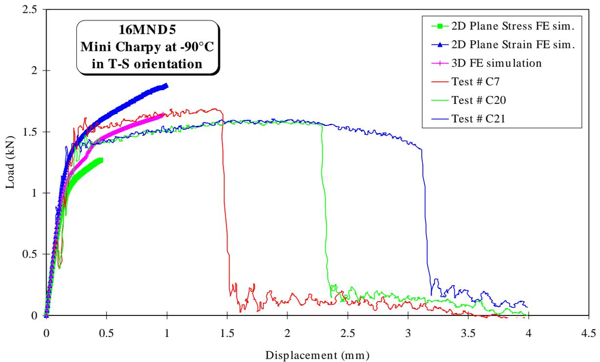
**Figure 5 :** Comparison of experimental and simulated (2D and 3D) load versus displacement curves for Sub-Size Charpy specimen at  $-90^{\circ}\text{C}$ .
