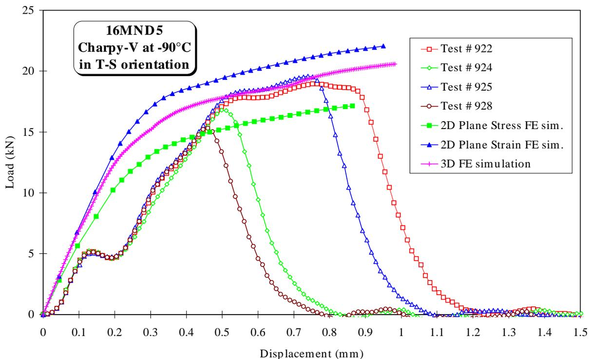
Figure 4 : Comparison of experimental and simulated (2D and 3D) load versus displacement curves for Charpy-V specimen at  $-90^{\circ}\text{C}$ .
