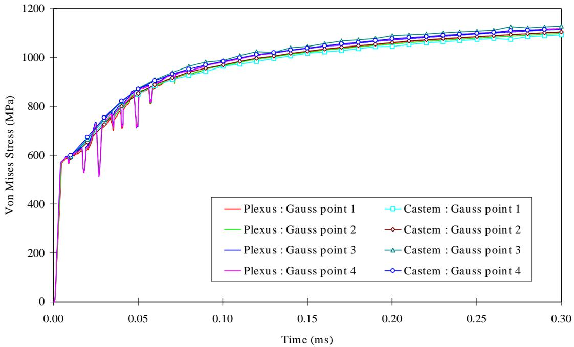
**Figure 2 :** Comparison between dynamic and quasi-Static 2D plane strain FE simulations of Sub-Size Charpy at  $-90^{\circ}\text{C}$ .
