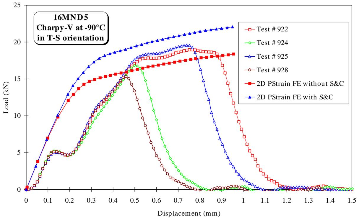
Figure 3 : Influence of strain rate on the global mechanical response for Charpy-V at  $-90^{\circ}\text{C}$ .
