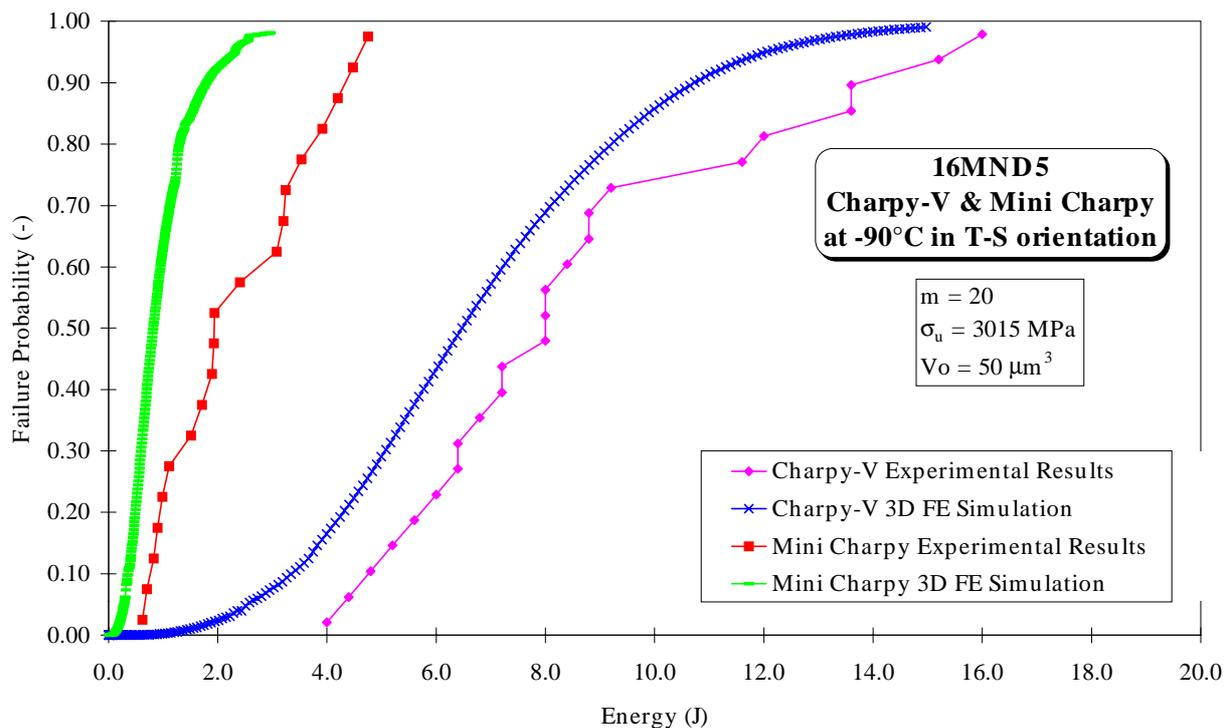
Figure 6 : Experimental and calculated cleavage failure probability for Charpy-V and Sub-Size Charpy.
