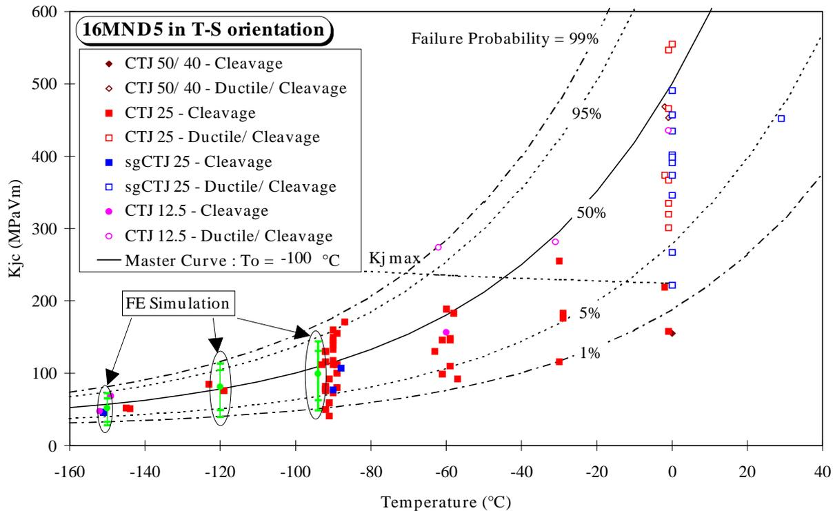
Figure 7 : Master curve and position of CT 25 finite element simulations.
