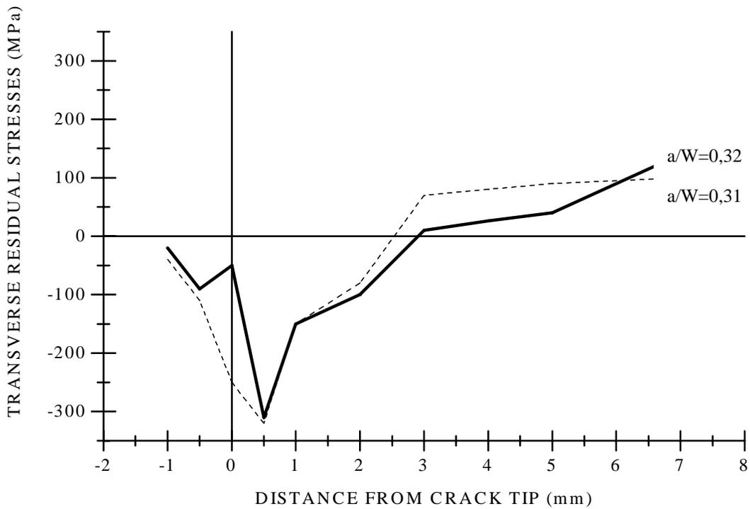
**Figure 2:** Residual stress distribution on the specimens' surfaces after consecutive overload cycles at different intervals of crack propagation. Both overloading ratios were equal to 2.
