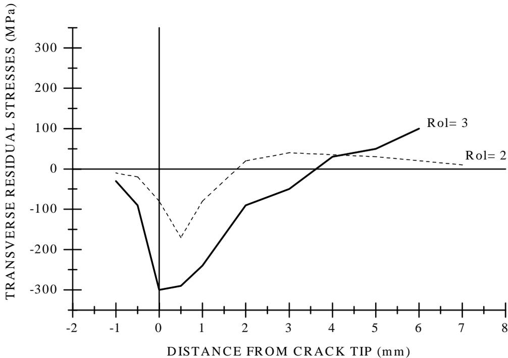
**Figure 1:** Residual stress distribution on the specimens' surfaces after single overload cycles.
