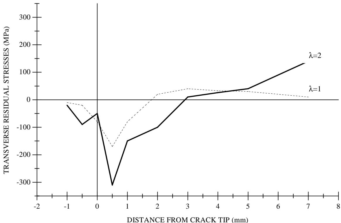
**Figure 3:** Residual stress distribution on the specimens' surfaces after single ( $\lambda=1$ ) and consecutive ( $\lambda=2$ ) overload cycles with the selected overloading ratios equivalent to 2.
