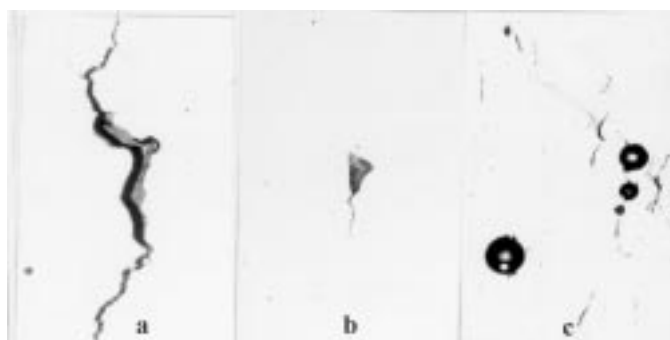
Figure 2: Microcracks initiation near inclusions of type two (a), type three (b) and type one (c).
