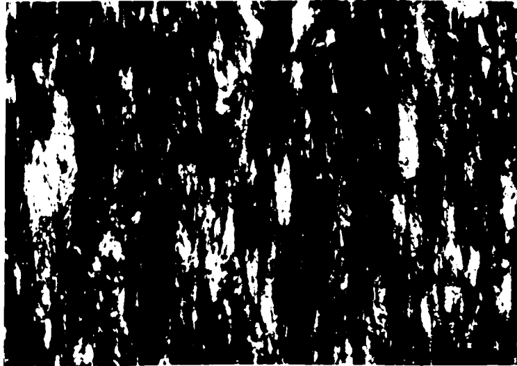
Figure 1: Optical micrograph of the longitudinal metallographic section showing the first microstructural level, i.e., the pearlite colonies oriented after cold drawing (vertical side: wire axis or cold drawing direction).
