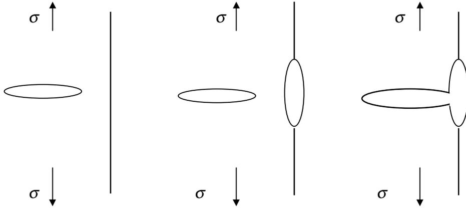
Fig.1: Crack arrestor formed by an interface
