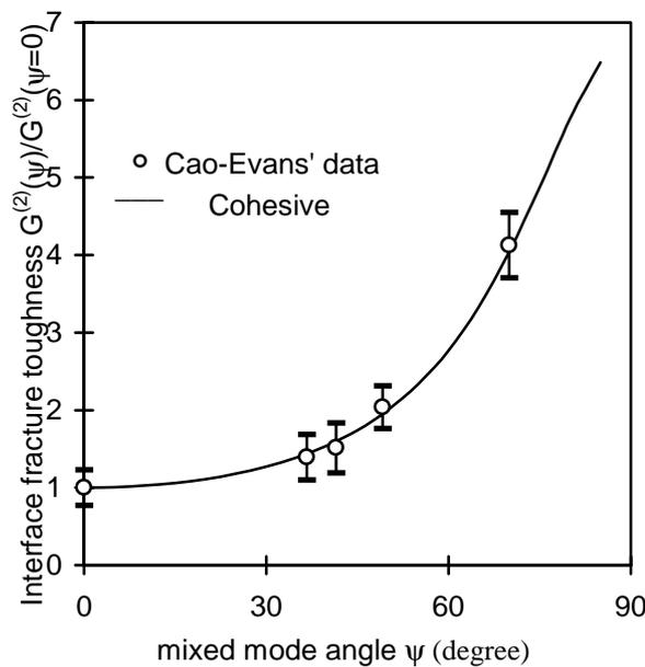
Figure 5 : Comparison of the Cao-Evans data for an epoxy/glass interface with the adhesive model for  $\sigma_c/\tau_c = 1/7$
