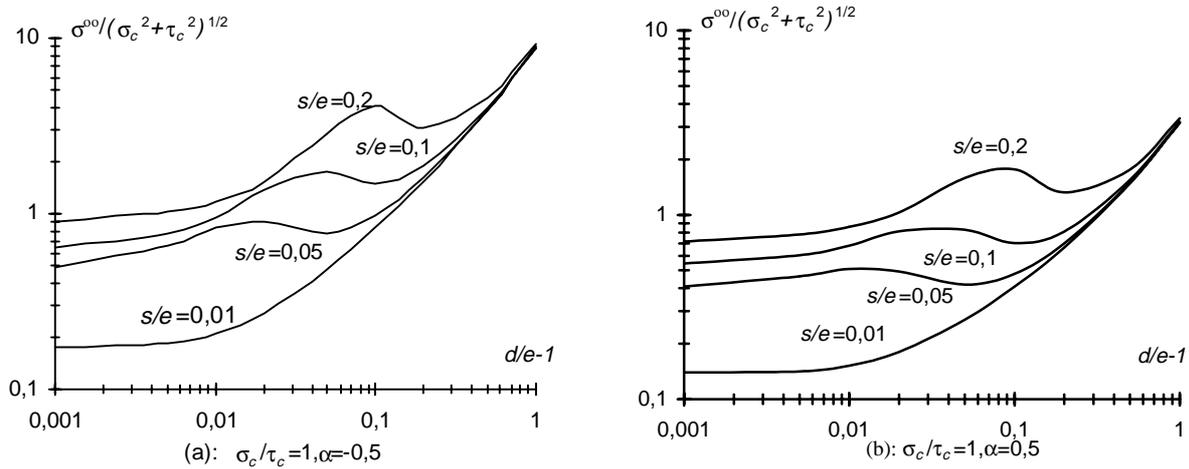
Figure 7: Critical remote tensile stress for interface debonding,  $\sigma_c/\tau_c = 1$
