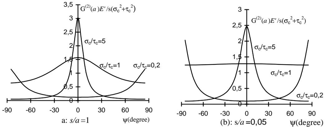
Figure 4 : Interface toughness as function of the mixed mode angle  $\psi$
