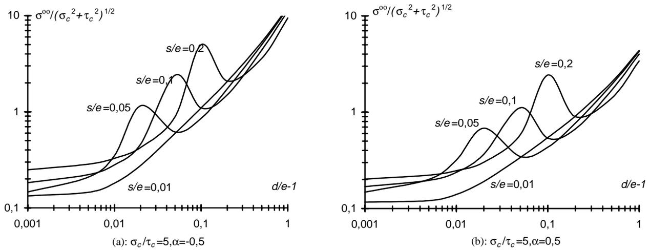
Figure 8: Critical remote tensile stress for interface debonding,  $\sigma_c/\tau_c = 5$
