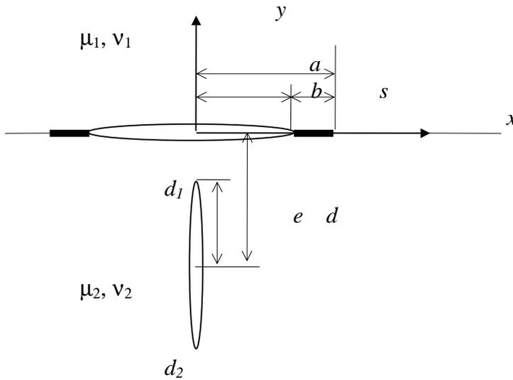
Fig.2: A crack normally approaching an interface and leading to interface debonding
