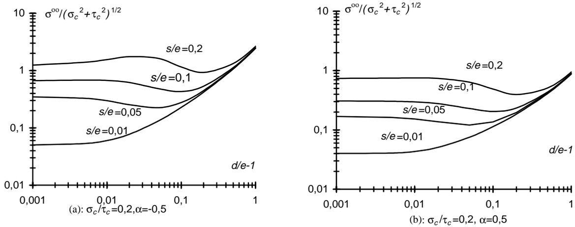
Figure 6: Critical remote tensile stress for interface debonding,  $\sigma_c/\tau_c = 0.2$
