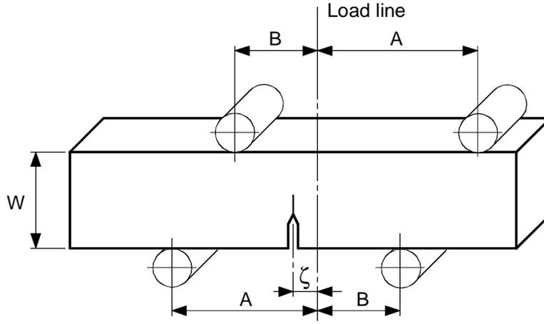
**Figure 1:** Experimental mixed-mode asymmetric four-point bend configuration.
