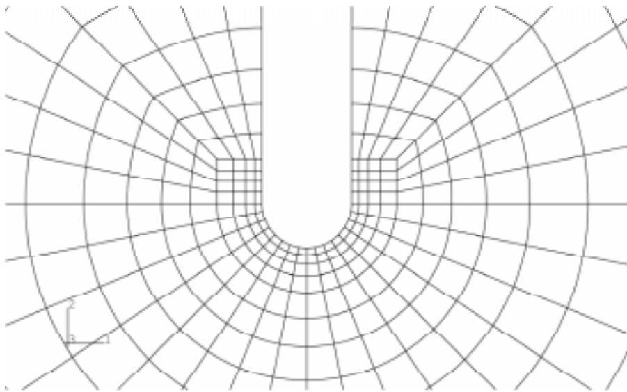
**Figure 2:** Near crack tip region finite element mesh of  $10 \times 10 \times 55 \text{ mm}^3$  specimen.
