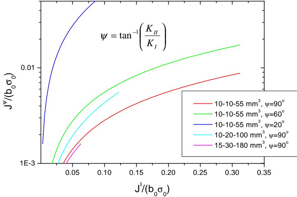
**Figure 6:** Scaling model results for different specimen sizes under mixed-mode I-II loading ( $b_0$  is the specimen ligament and  $\sigma_0$  a normalization stress, the proof stress).
