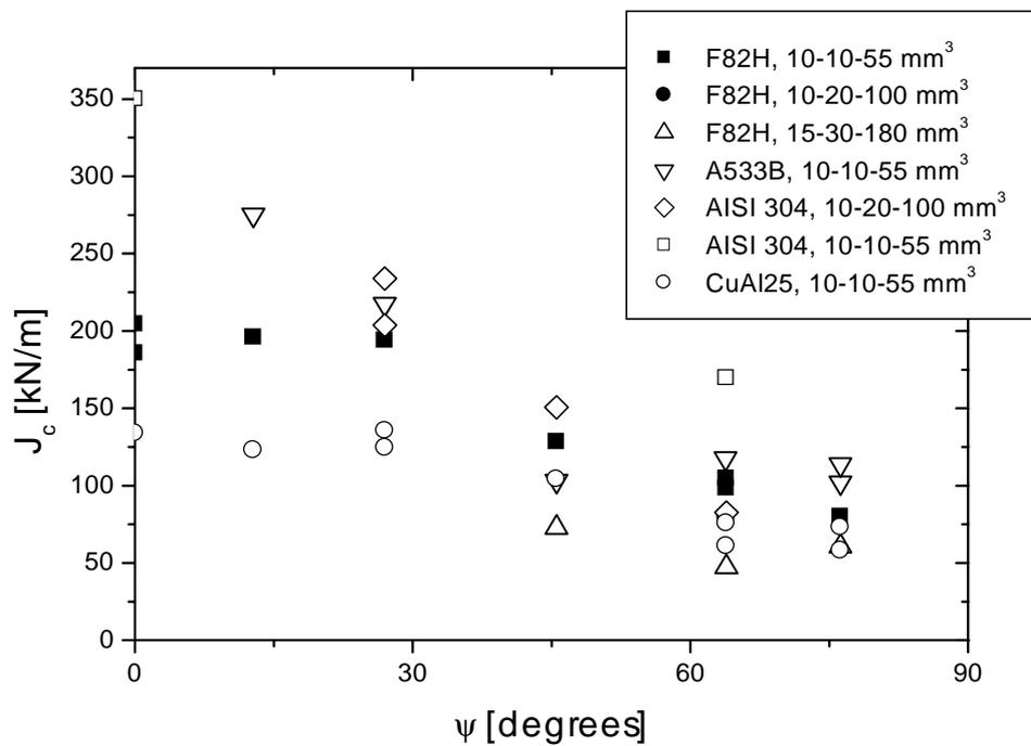
**Figure 3:** Transition of initiation toughness values in the mixed-mode I-II envelope.
