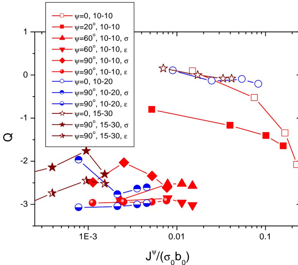
**Figure 7:** Values of Q-parameter as dependent on state of mixed-mode loading and specimen size.
