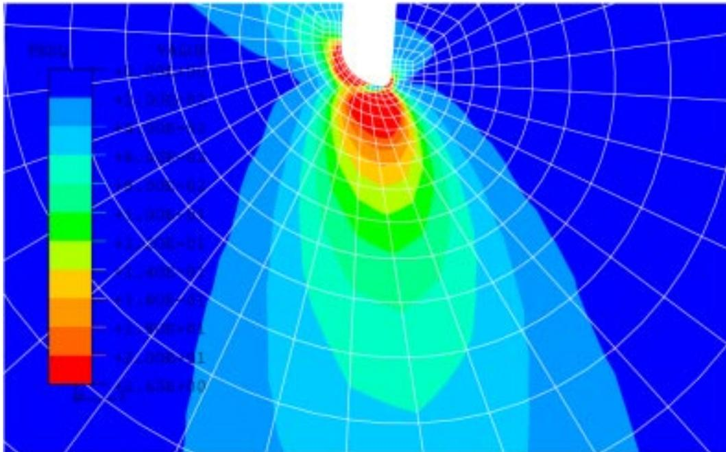
**Figure 5:** Distribution of equivalent plastic strain in the near tip regions of a CVN-size SENB specimen under mode II loading.
