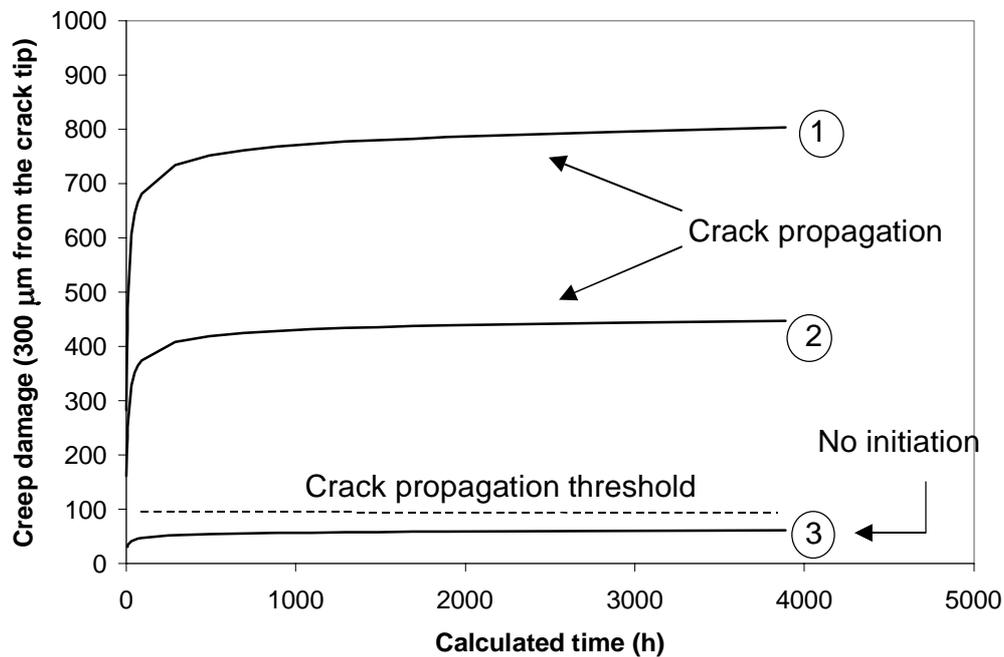
**Figure 4:** Level of creep damage at 300 μm from the tip of the crack of three CT specimens creep tested under various loads. Metallographic observations showed that the threshold identified was respected
