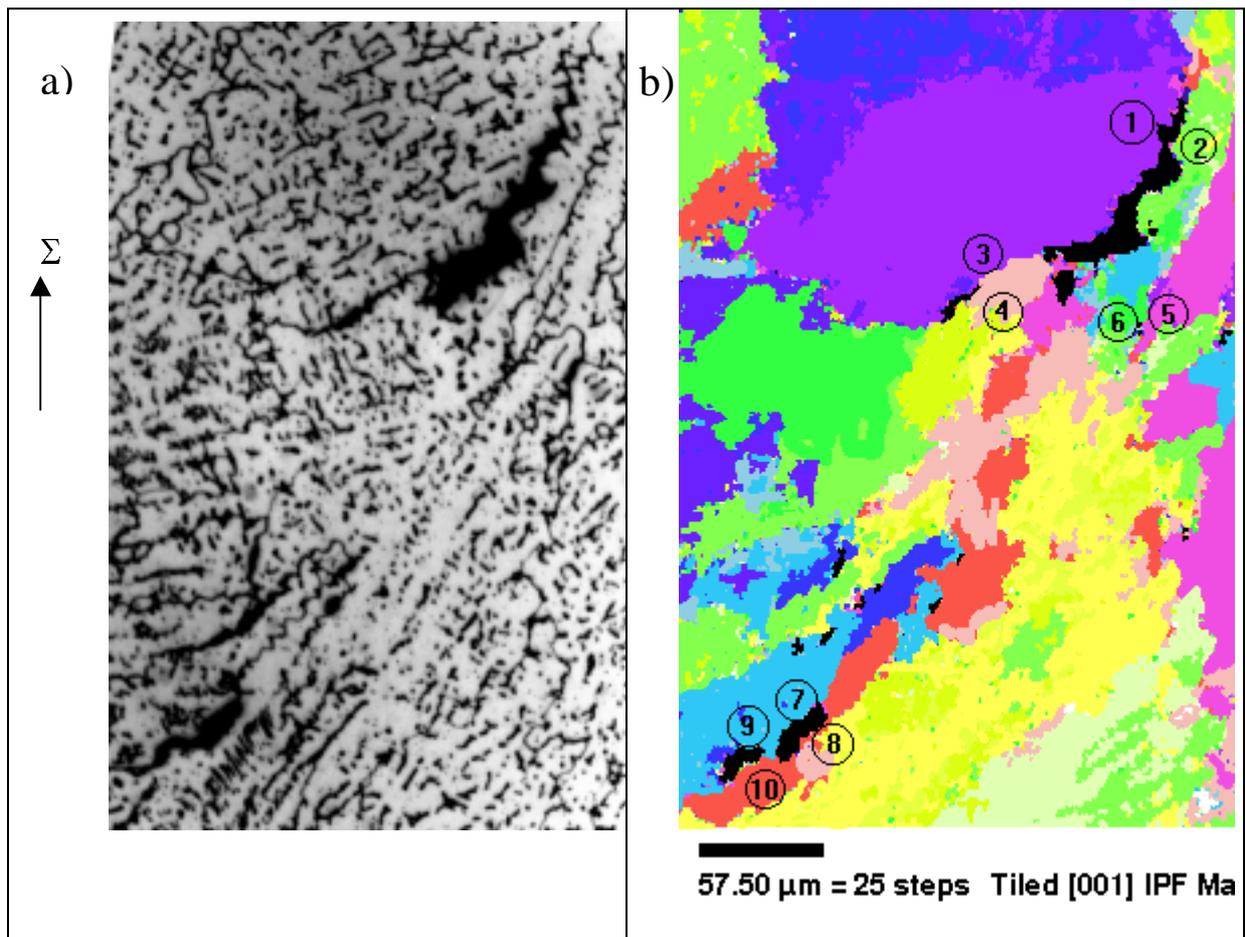
**Figure 3:** EBSD study of a damaged area
