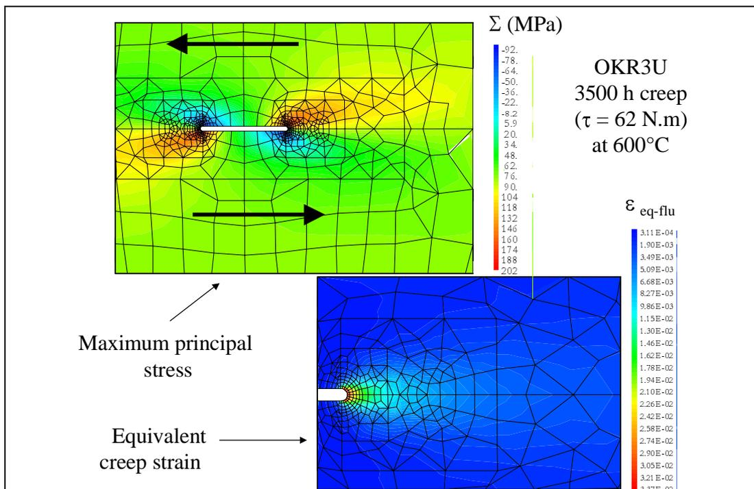
**Figure 6:** Notched plate under  $\tau = 62 \text{ N.m}$  at 600°C for  $t = 3500 \text{ h}$
