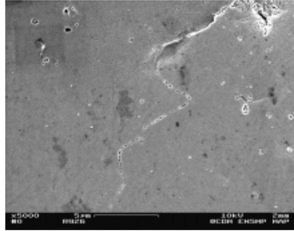
**Figure 2:** Creep cavitation at a grain boundary observed on a longitudinal section of a notched specimen
