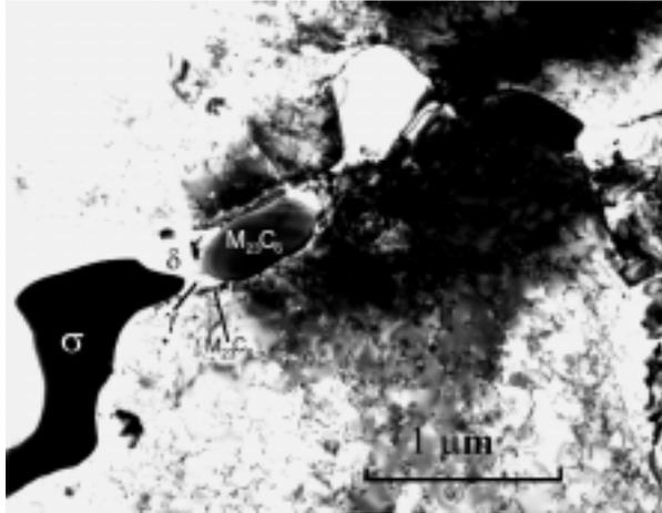
**Figure 1:**  $\sigma$  phase,  $M_{23}C_6$  and secondary  $\gamma$ -austenite. Material aged for 2000 h at 600°C
