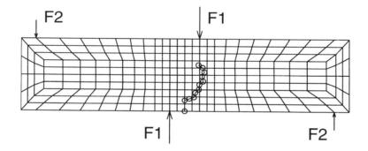
Figure 2: Crack pattern in single-edge notched beam loaded under shear conditions. Crack is initiated at bottom edge of beam.
