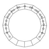
Figure 4: Crack pattern in hollow cylindrical pipe loaded by torsional moments. (b) Cross-sectional view.
