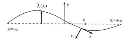
Figure 1: Geometry of curved crack.
