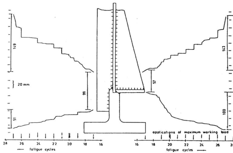
Figure 1 Variation of crack growth in the bridge girder stem with fatigue cycles
