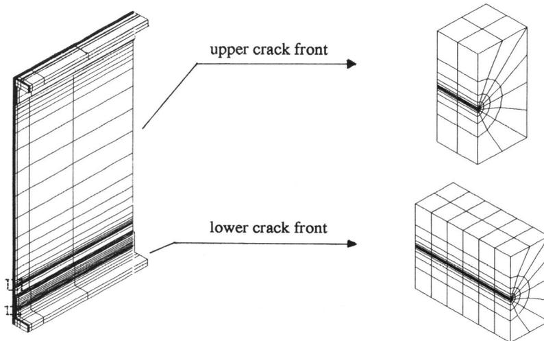
Figure 2 Typical three-dimensional finite element model containing through-thickness stem crack, lower and upper crack fronts are enlarged.
