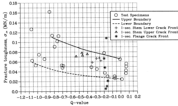
Figure 4 Variation of the fracture toughness with the Q-value for the test specimens. The  $J$  values of the I-section girder containing cracks are shown
