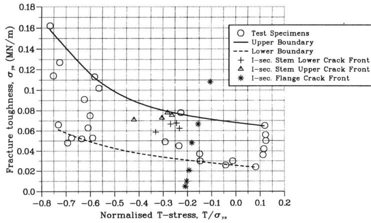
Figure 3 Variation of the fracture toughness with the normalised T-stress for the test specimens. The  $J$  values of the I-section girder containing cracks are shown
