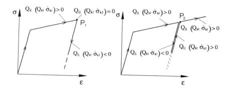
Fig. 3: Transition condition for  $\theta_{\text{pl}}$
