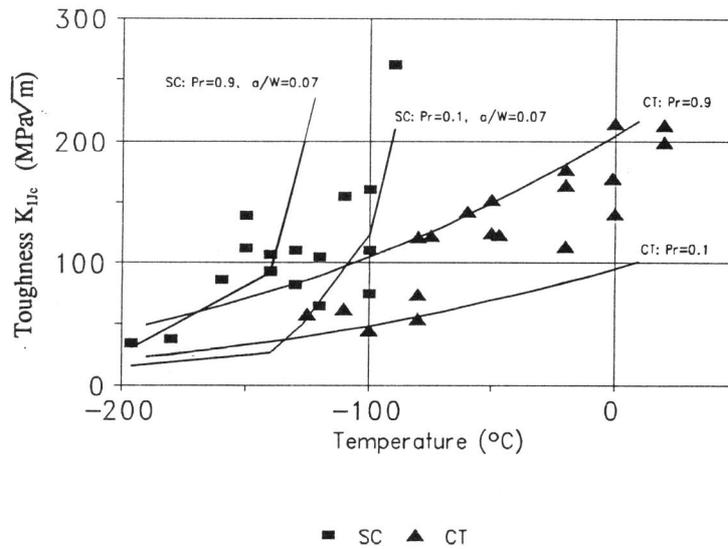
Figure 5: Transition temperature shift due to the shallow crack (SC) effect ( $a/W=0.07$ ). The probabilities to failure of  $Pr=0.1$  and  $Pr=0.9$  are indicated.
