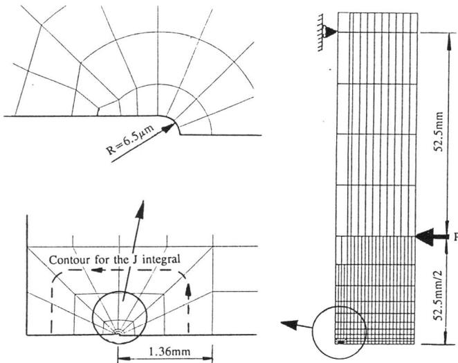
Figure 3: FE-mesh used for modelling the shallow crack specimen T84-10
