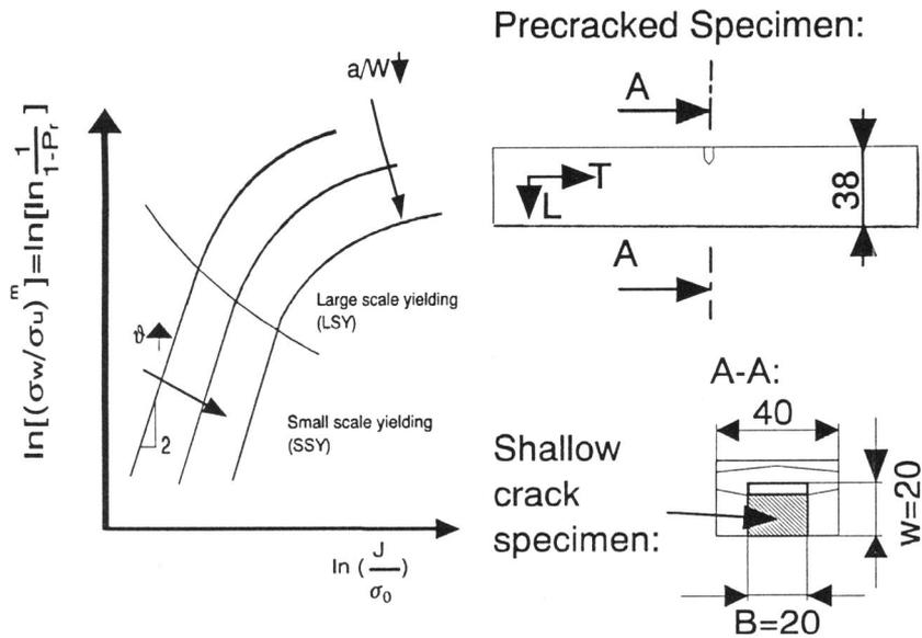
Figure 1: Loss of constraint effect ( $a/W \downarrow$ ,  $\vartheta \uparrow$ ) in a Weibull diagram
