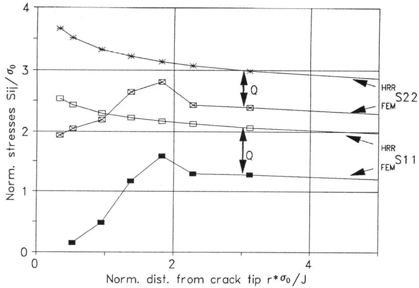
Figure 4: Stress distribution at the crack tip modelled with a finite initial radius of  $6.5\mu\text{m}$  (specimen T84-10)
