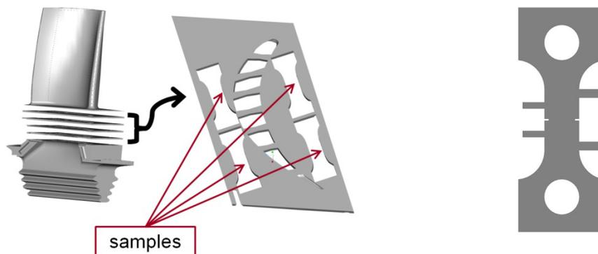
Figure 1: Positioning of specimen within a blade and specimen with notch
